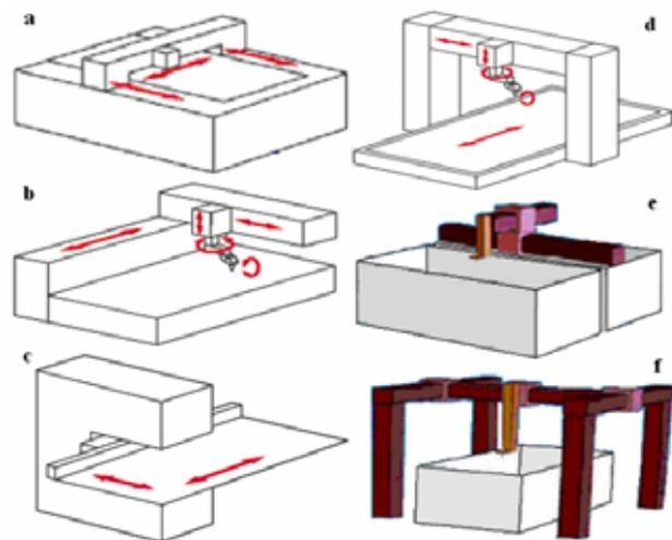
Fig. 1. Types of the positioning structures.
