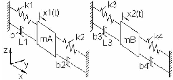
Fig. 4. Dual mass model of the parallel structure
