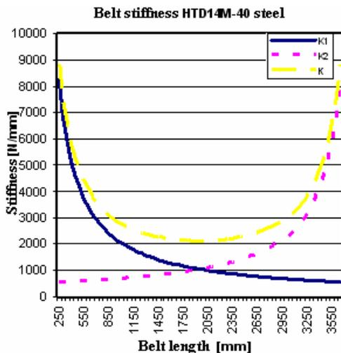
Fig. 9. Stiffness of the tooth belt drive.
