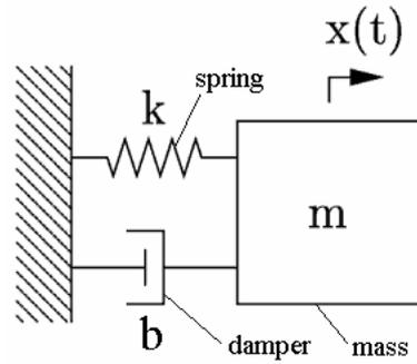
Fig. 3. Mass-spring-damper model.
