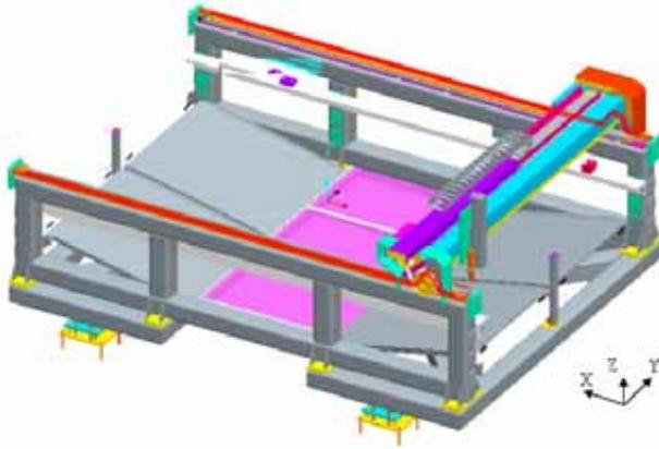
Fig. 7. Mechanical structure with parallel drives.
