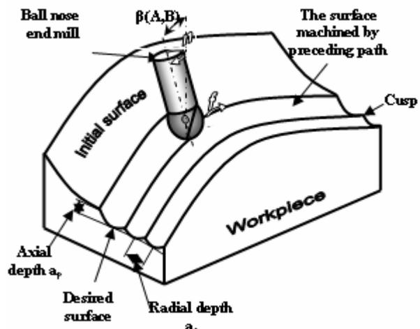
Fig. 1. Ball nose end milling process in 5 axes.
