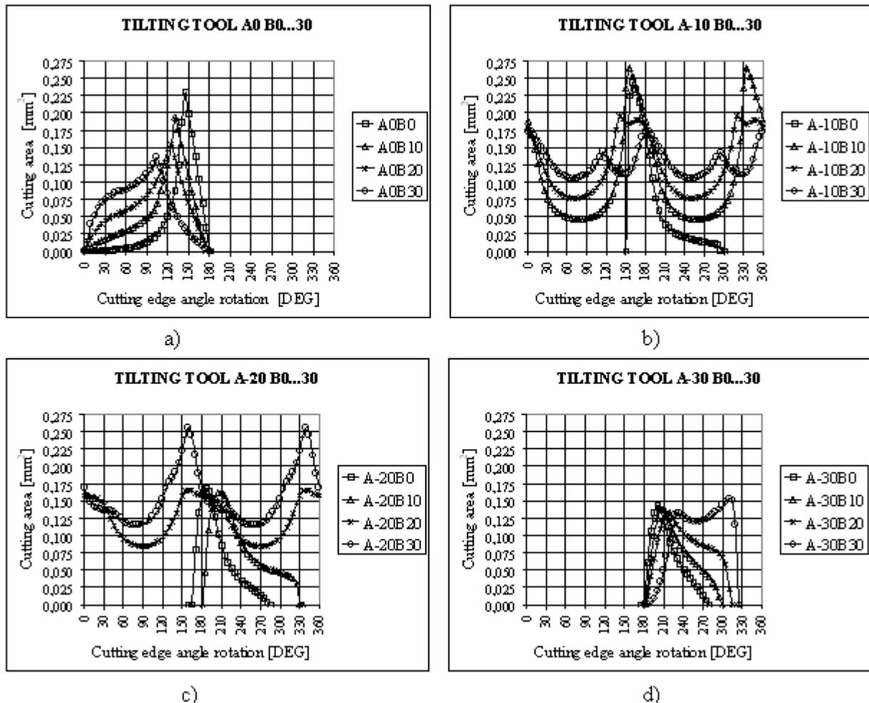
Fig. 6. Cutting area for different tilted tool position in second quadrant.
