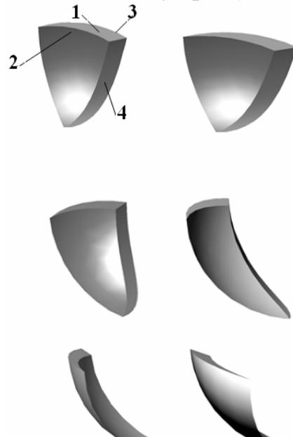
Fig.3. Different side views of uncut chip.
