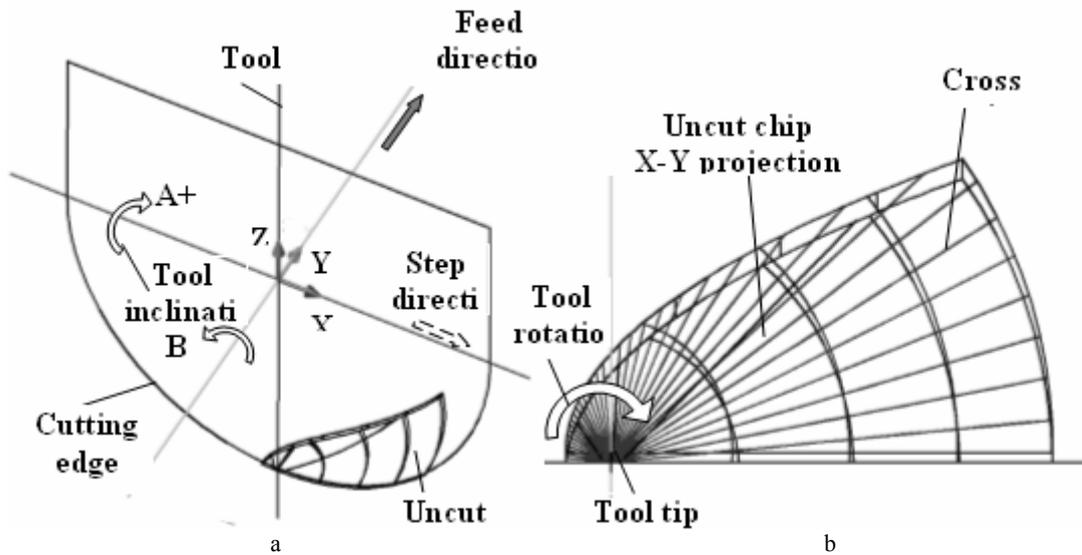
Fig. 4. CAD study of uncut chip cross sections (tilting tool A0B0).
