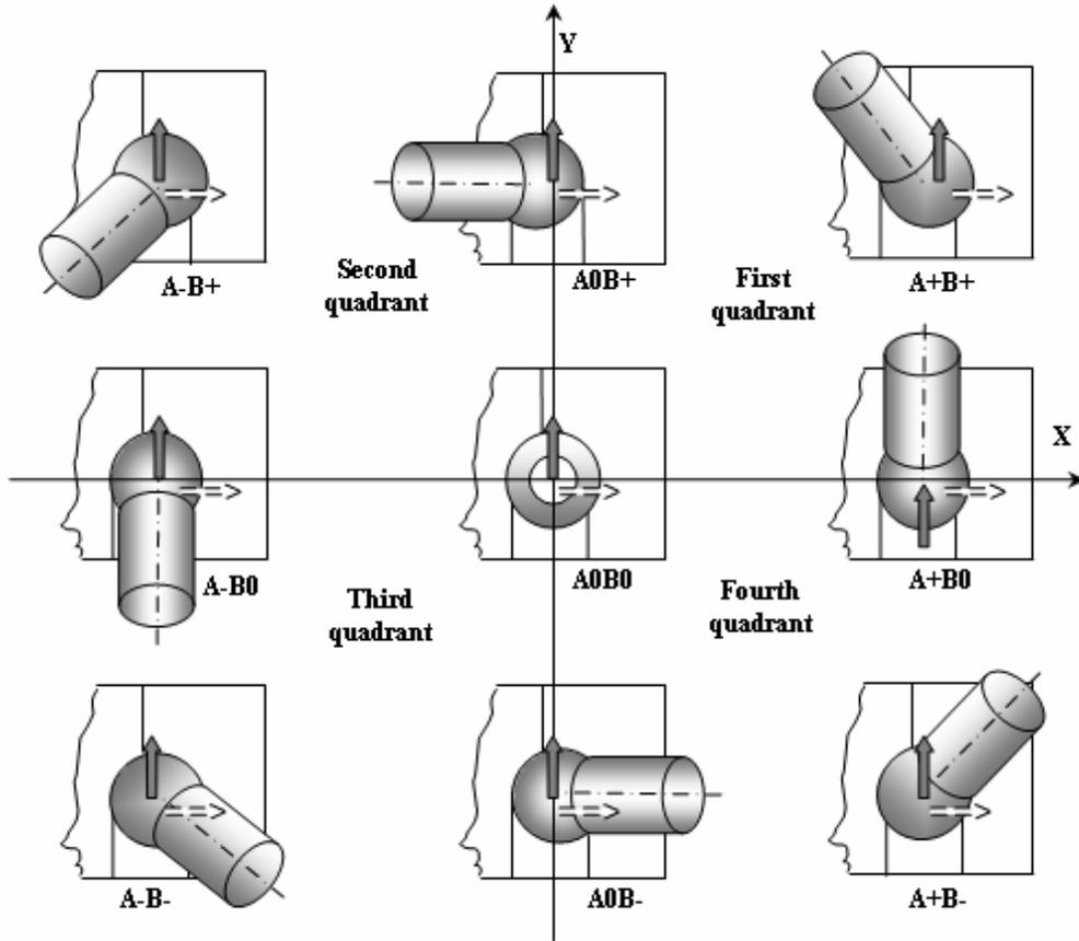
Fig. 2. Tilted tool position in 5 axes machining.
