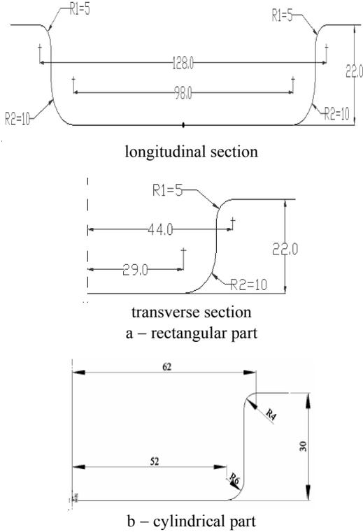
Fig. 2. Geometry of the drawn parts.
