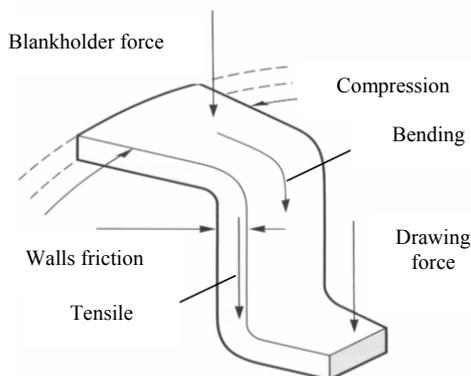
Fig. 1. Efforts that stress the material during deep drawing.
