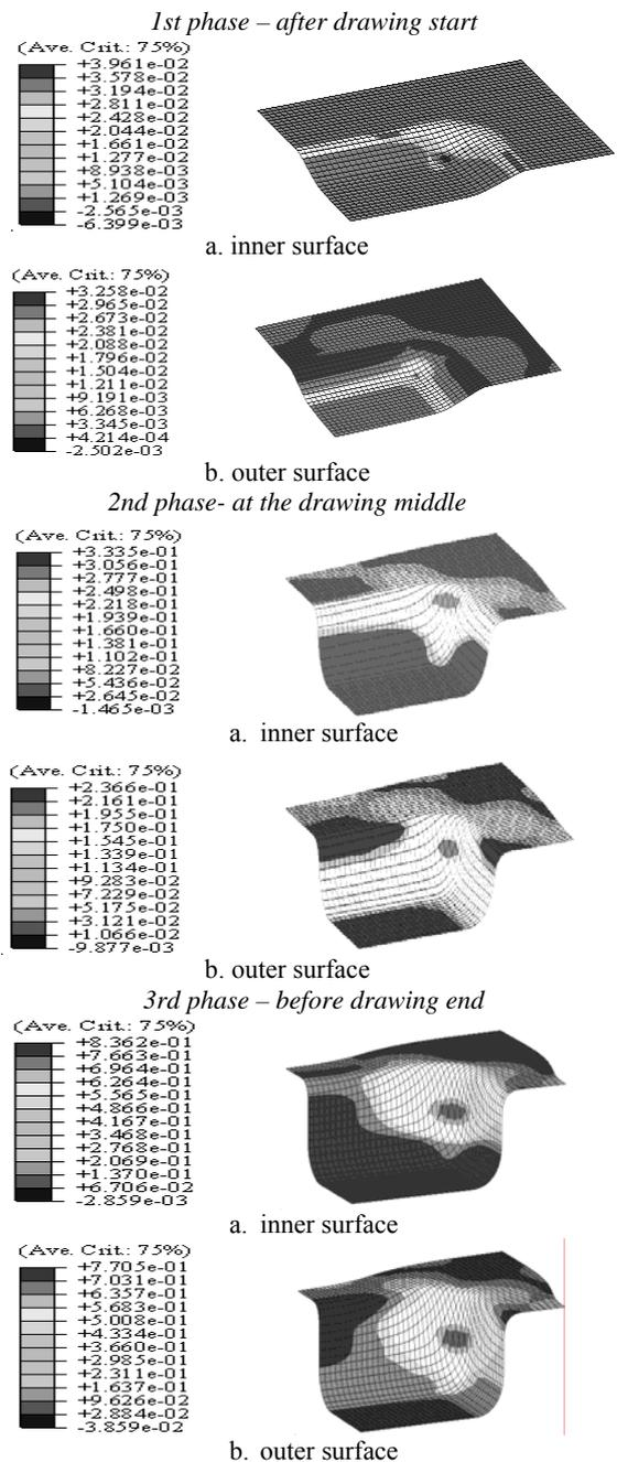
Fig. 4. Strains analysis in the case of rectangular part.
