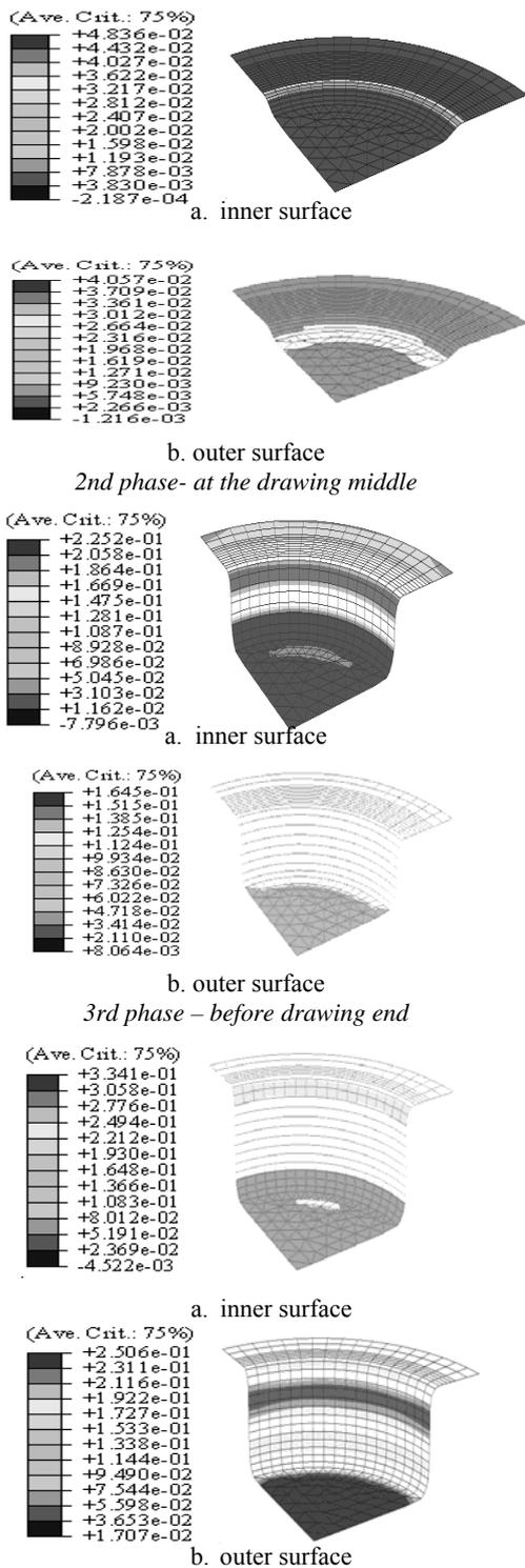
Fig. 5. Strains analysis in the case of circular part.
