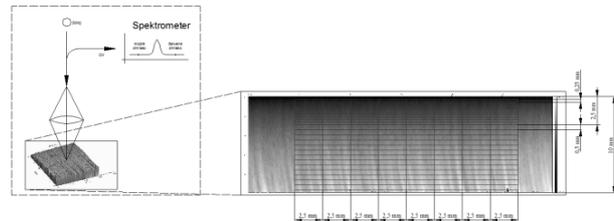
Fig. 4. Depth traces in which have been detected quantitative surface profile roughness parameters  $R_a$ ,  $R_q$  and  $R_z$ .
