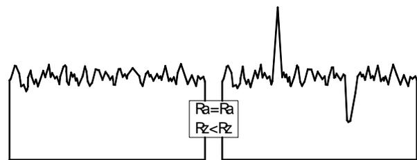
Fig. 3. An illustrative example of two equal surfaces in terms of parameter roughness profile  $R_a$ , but different in terms of the surface profile roughness parameter  $R_z$ .
