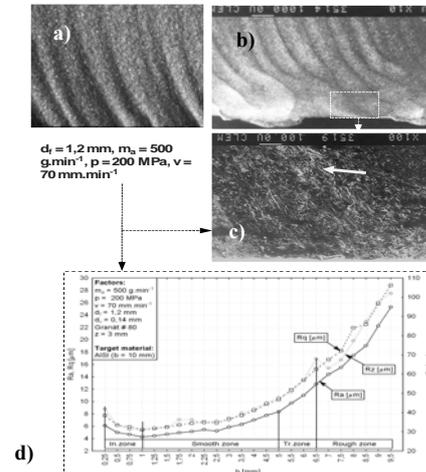
Fig. 5. a) surface produced from AISI 304 under defined conditions  $d_f = 1,2$  mm,  $p = 200$  MPa,  $m_a = 500$  g.min<sup>-1</sup> and  $v = 70$  mm.min<sup>-1</sup>, b) SEM photograph of surface 10x, c) surface detail with visible grooving and plastic deformation, d) topographic function including of initial zone.
