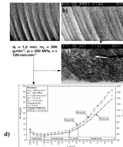
Fig. 6. a) surface produced from AISI 304 under defined conditions  $d_f = 1,2$  mm,  $p = 350$  MPa,  $m_a = 300$  g.min<sup>-1</sup> and  $v = 120$  mm.min<sup>-1</sup>, b) SEM photograph of surface 10x, c) surface detail with visible grooving and plastic deformation, d) topographic function including of initial zone.
