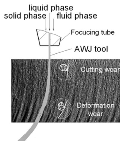
Fig. 1. Abrasive waterjet surface creation.
