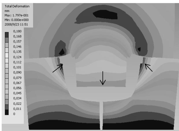
Fig. 8. Total deformation – Alumecc,  $F = 200$  t.
