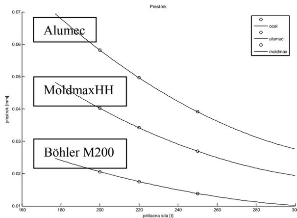
**Fig. 11.** Influence of pressure force on gap in division plane.
