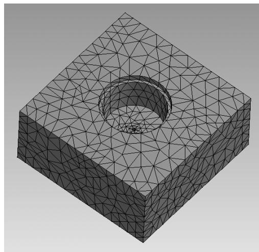
Fig. 5. Model mesh of lower part.
