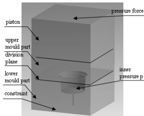
Fig. 1. Model and boundary conditions.
