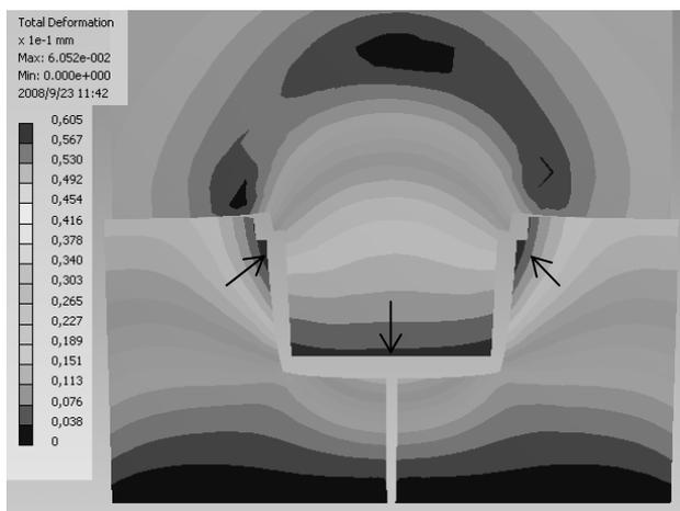
Fig. 7. Total deformation – Böhler M200,  $F = 200$  t.
