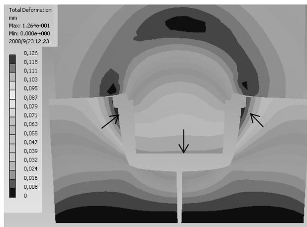
Fig. 9. Total deformation – MoldmaxHH,  $F = 200$  t.
