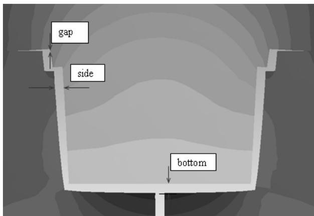
Fig. 6. Places of evaluation of displacements (zoom 50-times).
