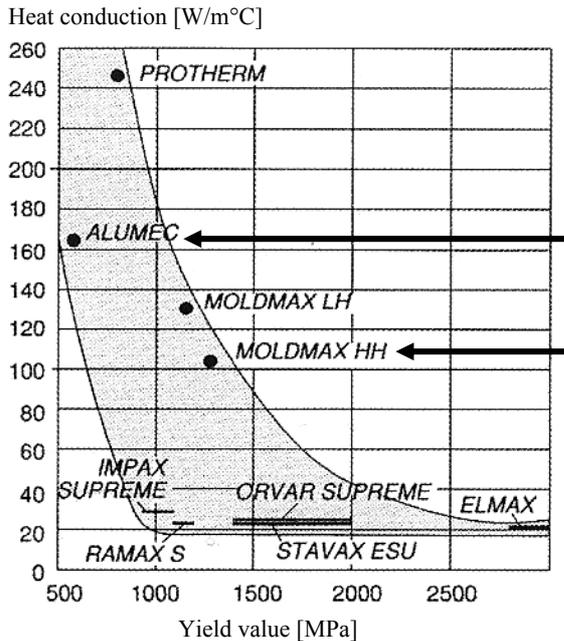
Fig. 3. Materials of mould.
