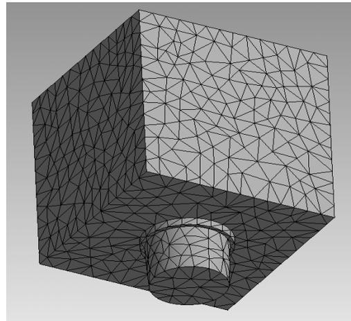
Fig. 4. Model mesh of upper part.
