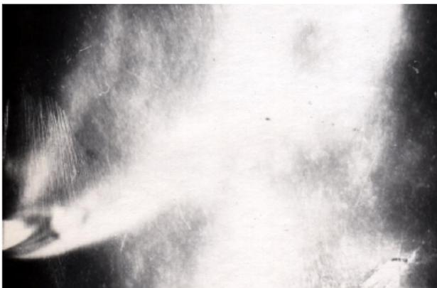
Fig. 7. The supersonic jet shown with a strong transversal flux.
