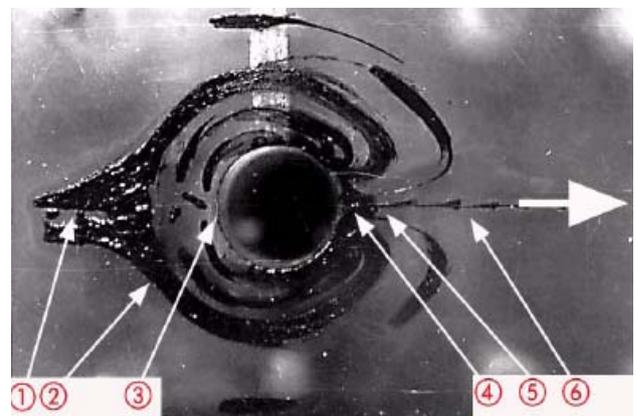
**Fig. 11.** Definition of the peripheral turbulence area of the supersonic jet.
