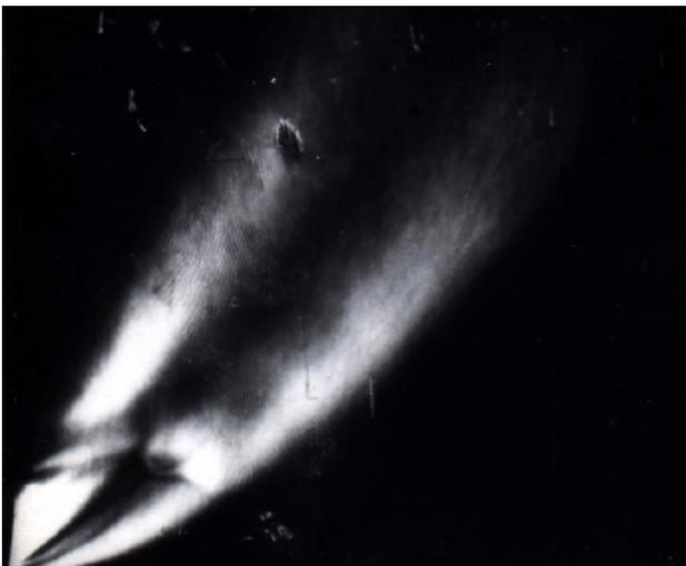
**Fig. 9.** The supersonic jet with a transversal flux, presenting a collision area.
