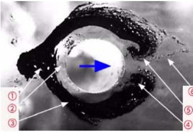
Fig. 12. Stagnation area in front of the Venturi's orifice.
