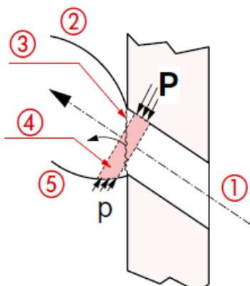
Fig. 3. The sonic line positioned perpendicular on the nozzle's axe. Legend: 1 – nozzle's axe; 2 – the profile of the under-expanded jet; 3 – the sonic line; 4 – the frontal area of the jet, at the nozzle's arrangement; 5 – the inferior limit layer of the jet.
