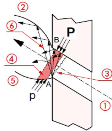
Fig. 4. The sonic line placed in the output plane of the jet. Legend: 1 – 5 as in Fig. 4; 6 – the interfered choke wave, generated by the A edge.
