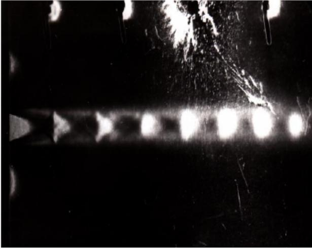
Fig. 5. Supersonic jet, without transversal flux, with expansion in the form of bell.
