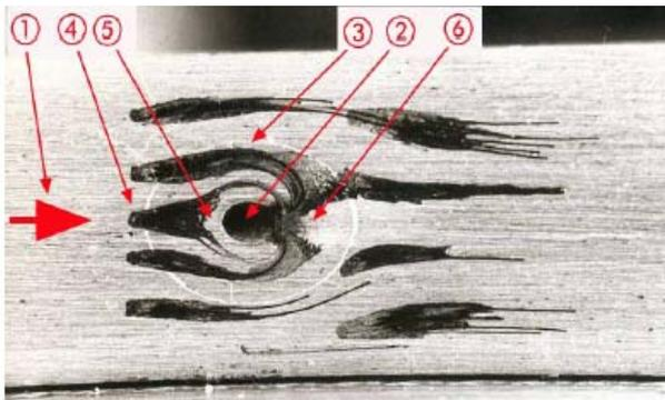
Fig. 13. Anterior and posterior turbulence areas of the supersonic jets.
