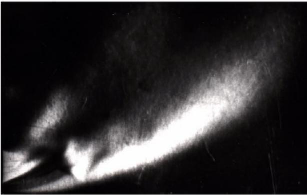
**Fig. 8.** The supersonic jet shown with a transversal flux; it can be seen the entrainment tourbillions.
