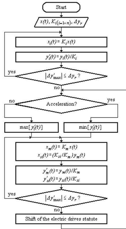
Fig. 3. Flowchart of the control algorithm.
