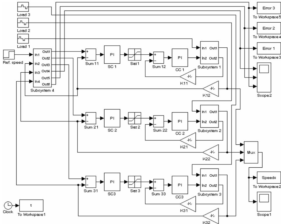
Fig. 4. Simulation model of a multi-motor electromechanical system.
