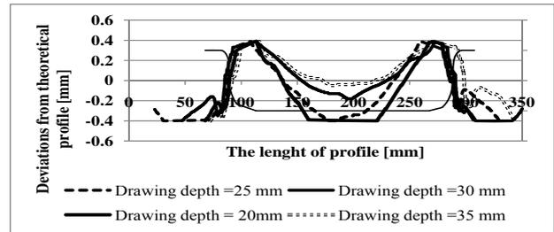
Fig. 9. Deviations from theoretical profile on diagonal sections.
