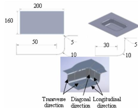
Fig. 1. Part geometry and analyzed sections.
