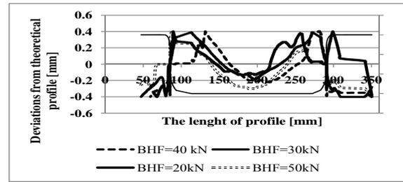
Fig. 6. Deviations from theoretical profile on diagonal sections.
