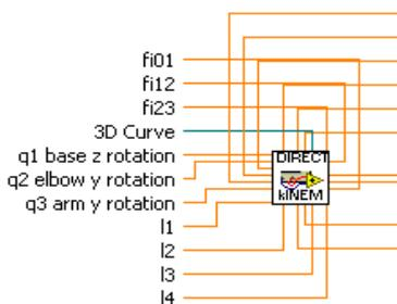
Fig. 4. The icon of the LabVIEW VI for the assisted simulation of the direct kinematics.
