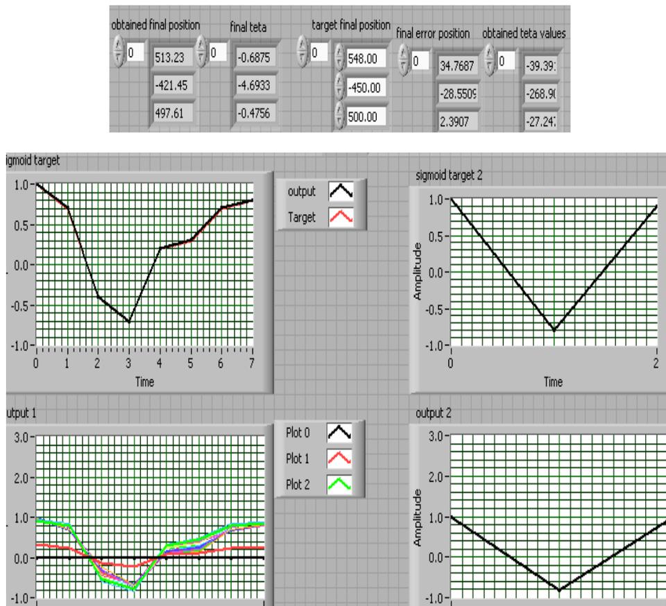
**Fig. 15.** The front panel of the VI with the target and obtained curves after applying the proper inverse kinematics neural network – case study 2.
