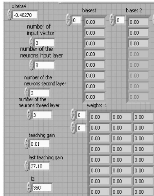
**Fig. 13.** Front panel with the input data concerning the number of neurons in each layer, teaching gains, initialized weights and biases matrices.
