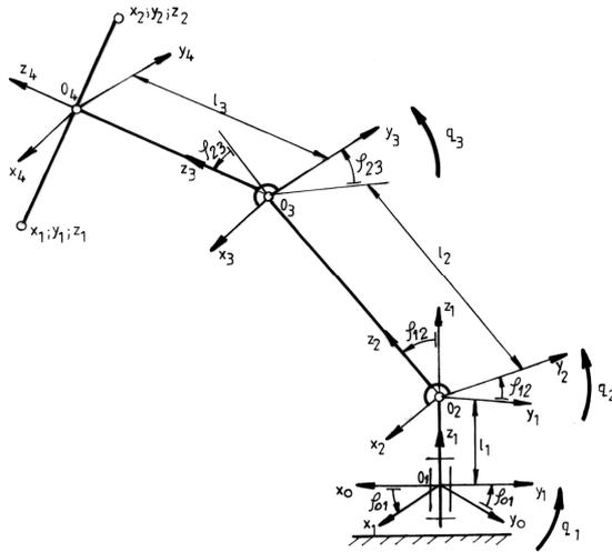
Fig. 2. The cinematic structural schema of the studied arm type robot.
