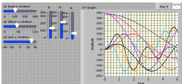
Fig. 3. The variation of the absolute coordinate functions of  $q_1, q_2$  or  $q_3$ .
