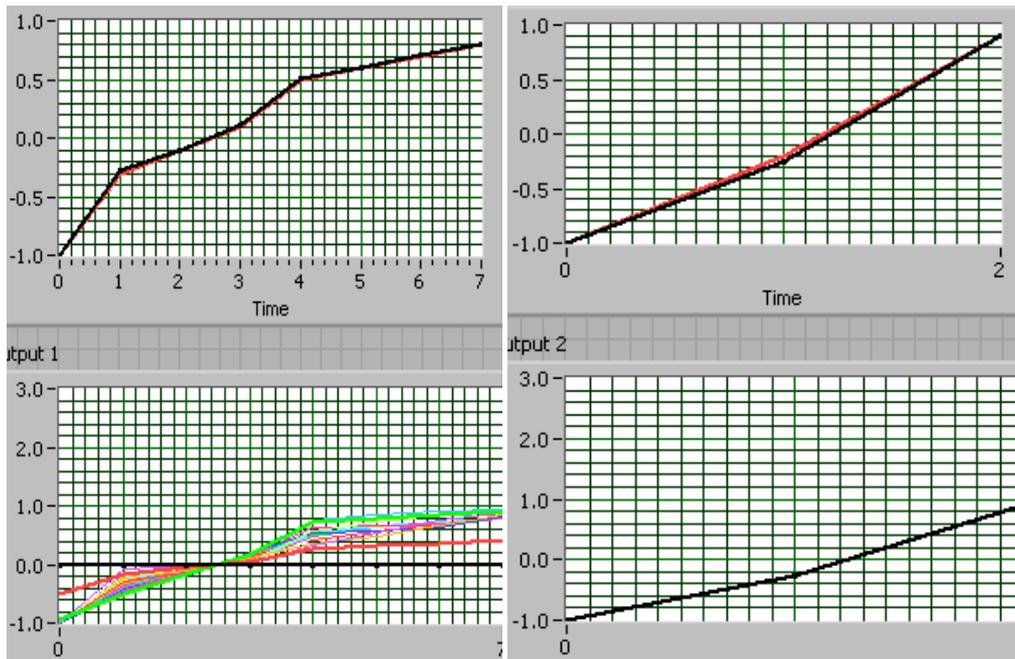
**Fig. 14.** The front panel of the VI with the target and obtained curves after applying the proper inverse kinematics neural network – case study 1.
