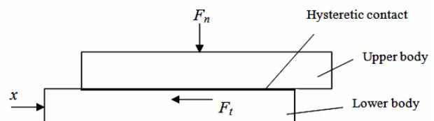
Fig. 1. Frictional contact of flat on flat connection.
