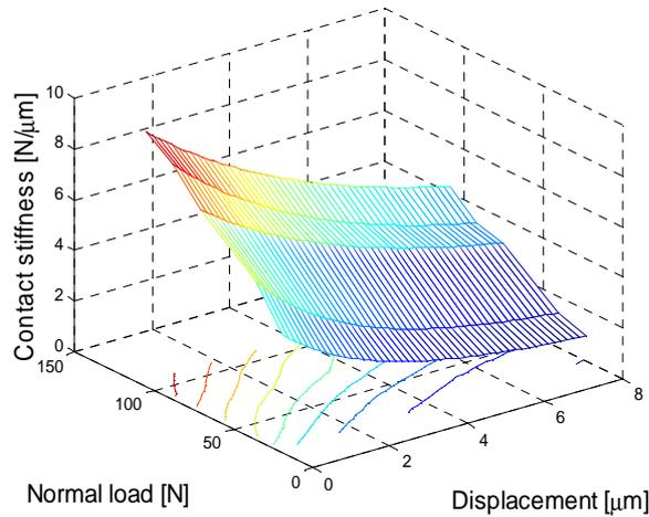
**Fig. 14.** Global stiffness in function of normal load and displacement.
