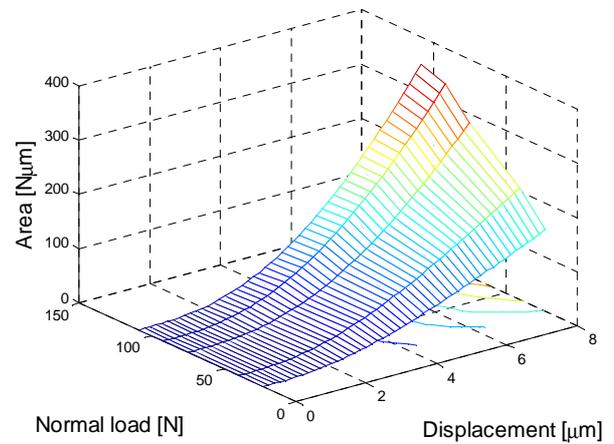
Fig. 11. Area in function of the normal load and displacement.
