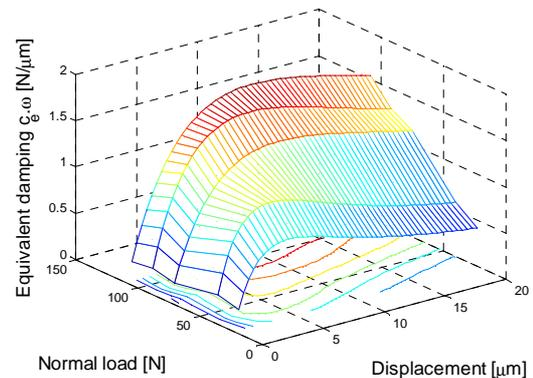
Fig. 12. Equivalent damping in function of normal load and displacement.
