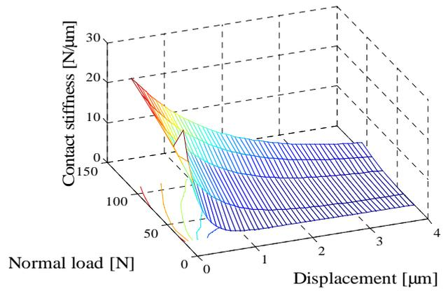
Fig. 9. Local stiffness as function of normal load and displacement.
