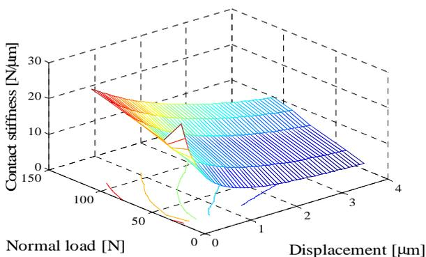
Fig. 8. Global stiffness as function of normal load and displacement.
