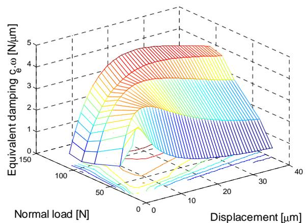
**Fig. 17.** Equivalent damping in function of normal load and displacement.
