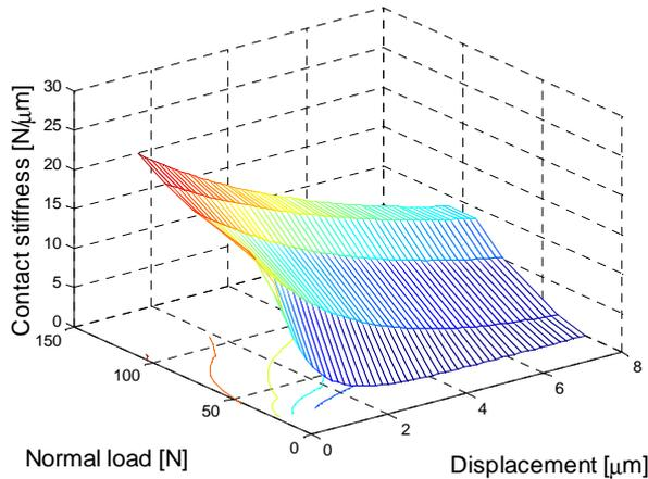
**Fig. 18.** Local stiffness in function of normal load and displacement.
