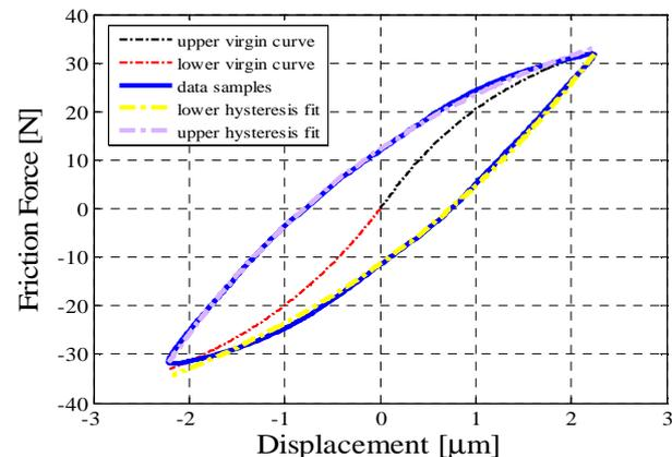
Fig. 5. Hysteresis in pre-sliding: Aluminum on aluminum,  $W = 109$  N,  $f = 1$  Hz.
