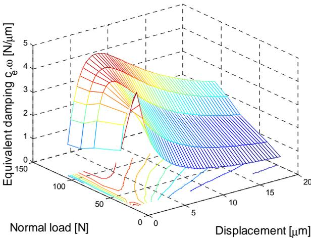
Fig. 7. Equivalent damping in function of normal load and displacement.
