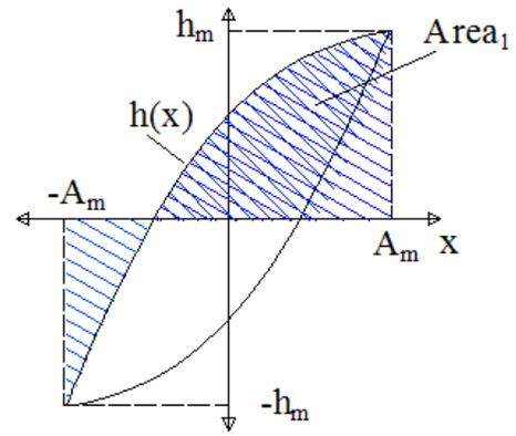
Fig. 3. Schematic representation of hysteresis area.
