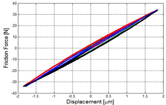
**Fig. 15.** Fitted hysteresis data:  $W = 75 \text{ N}$ ,  $f = 1 \text{ Hz}$ .
