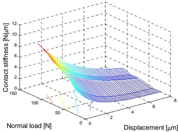
**Fig. 13.** Local stiffness in function of normal load and displacement.
