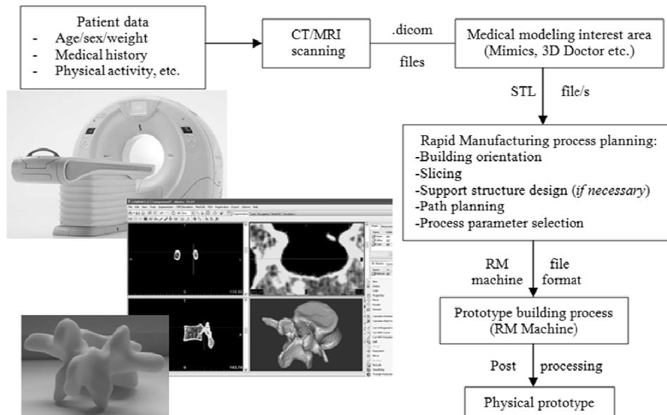
Fig. 1. Standard workflow for the design and rapid manufacturing of prototypes for medical applications.
