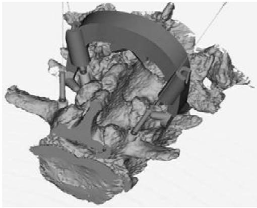
Fig. 3. Design of a guide for pedicle screws implantation [11].
