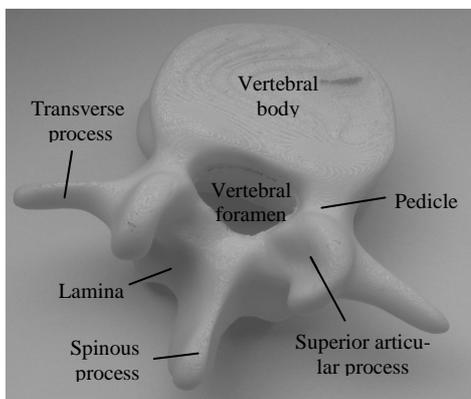
Fig. 2. FDM prototype of L3 vertebra.
