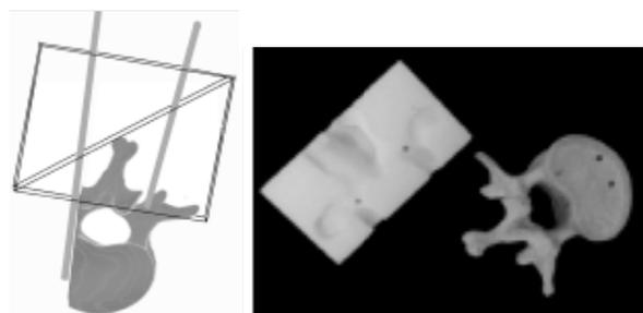
Fig. 7. Design of a block guide for pedicle screw insertion [17].
