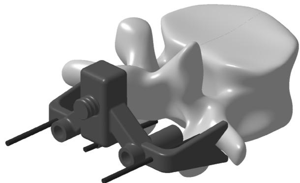
Fig. 10. Design of a drill guide for L3 vertebra.
