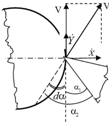
Fig. 5. Clearance angle variation  $d\alpha(t)$ .
