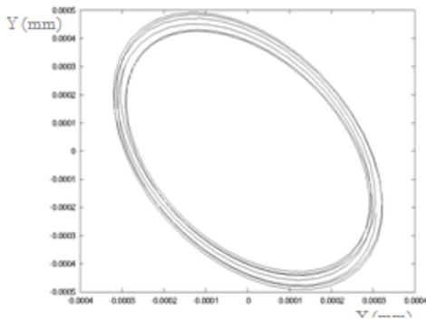
Fig. 7a. Trajectory of the tool tip ( $\theta = 48^\circ$  and  $F = 262.5$  Hz)
