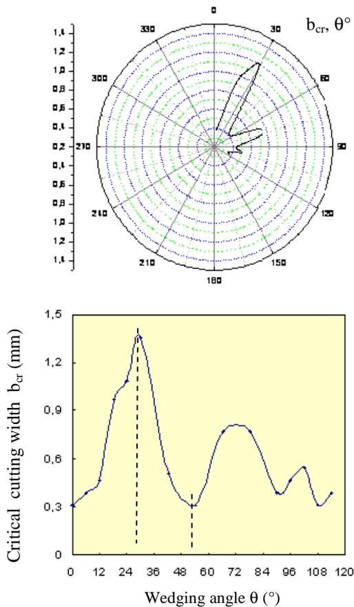
Fig. 11. Variation of cutting width.
