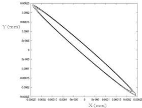
Fig. 7b. Trajectory of the tool tip ( $\theta = 30^\circ$  and  $F = 300$  Hz)
