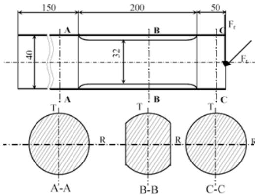
Fig. 1. Bar of unsymmetrical bending.
