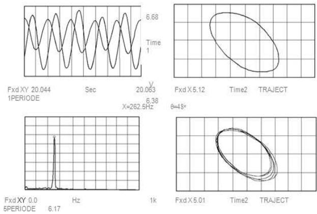
Fig. 12. Trajectory for  $\theta = 48^\circ$  and  $F = 262.5 \text{ Hz}$  and displacement  $Y = f(X)$ .
