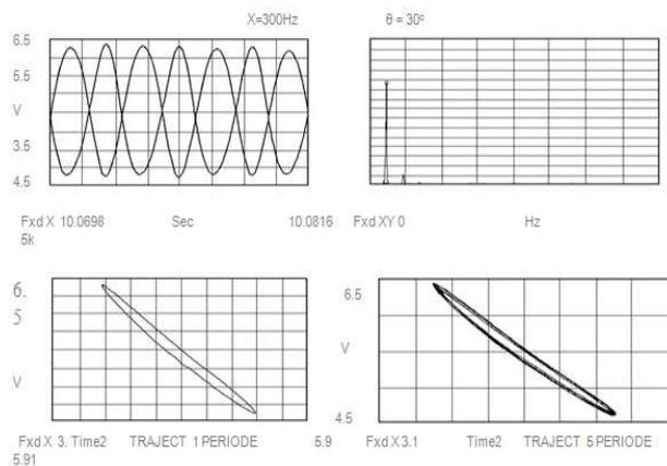
Fig. 13. Trajectory for  $\theta = 30^\circ$  and  $F = 300 \text{ Hz}$  and displacement  $Y = f(X)$ .
