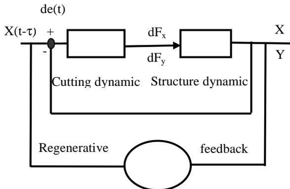
Fig. 3. Block diagram for regenerative chatter.
