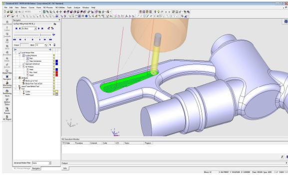
Fig. 7. Tool path for roughing.
