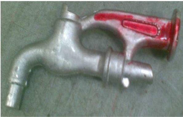
Fig. 13. Penetrant liquid application.
