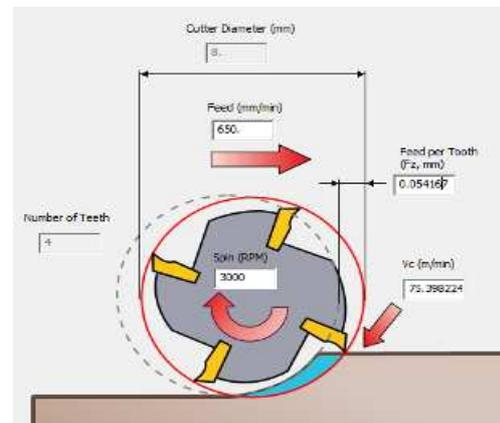
Fig. 6. Machining parameters.
