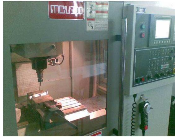
Fig. 10. Machining on MCV300 vertical milling center.
