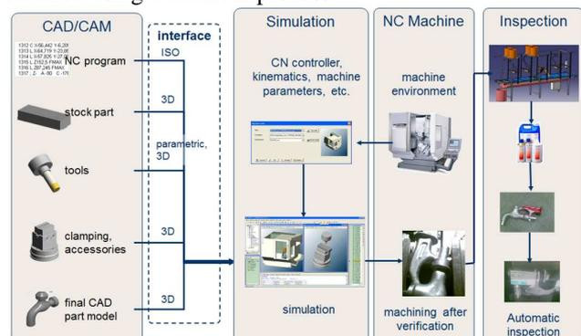
Fig. 1. General schema of general workpiece flow.
