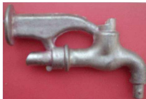
Fig. 4. Aluminium casting tap.
