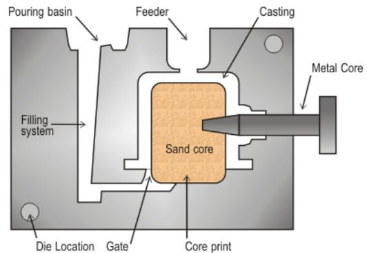
Fig. 2. Schematic view of a casting mould.
