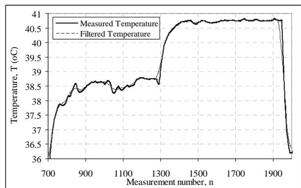
**Fig. 14.** Temperature monitoring of a working induction motor.
