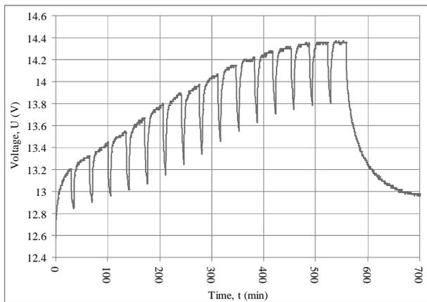
Fig. 15. Voltage monitoring of battery charge - discharge cycle.
