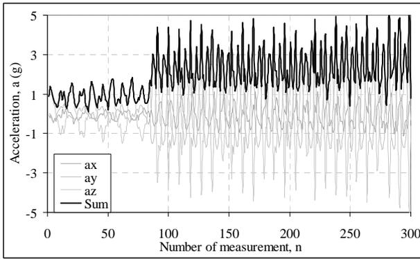
**Fig. 5.** Measured acceleration on all 3-axis and calculated amplitude of acceleration vector.
