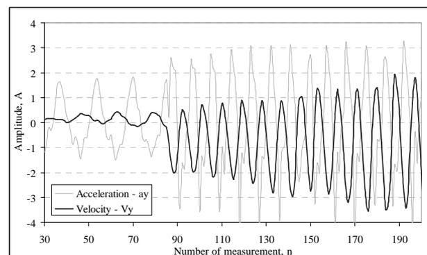
**Fig. 8.** Measured acceleration on y axis and calculated velocity.
