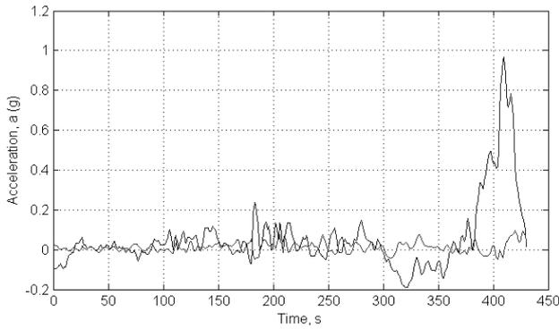
**Fig. 9.** Vibrations measured on X and Y axes of tested in-motion vehicle over a particular route.
