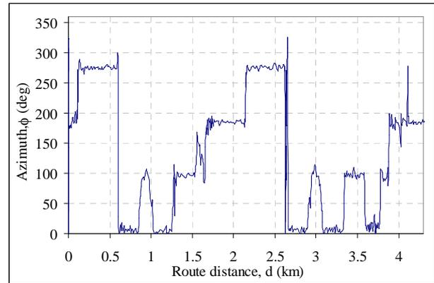
**Fig. 13.** Recorded motion direction in azimuth values of test vehicle in reference to the covered distance.
