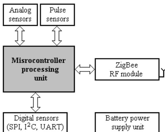
Fig. 3. Block diagram of the Zigbee measurement device.
