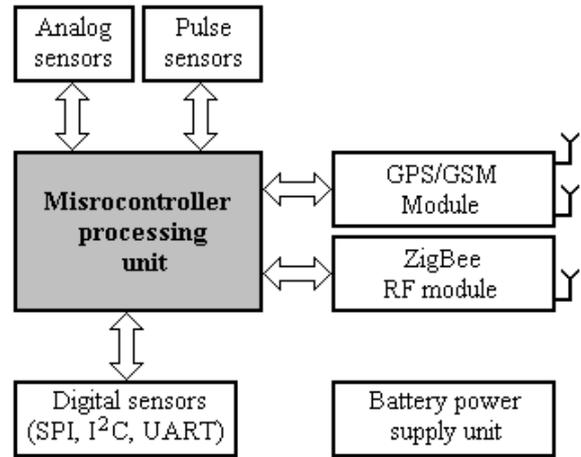
Fig. 2. Block diagram of Zigbee coordinator device.
