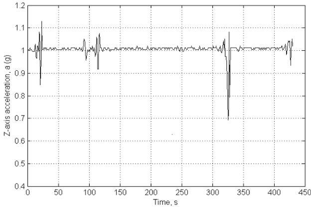
**Fig. 10.** Vibrations measured on Z axis of tested in-motion vehicle over a particular route.
