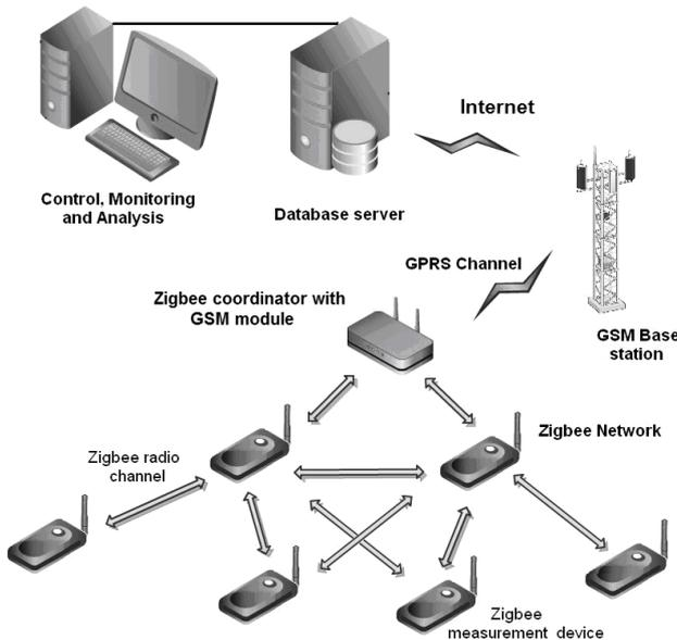
Fig. 1. Structure of the wireless measurement system.
