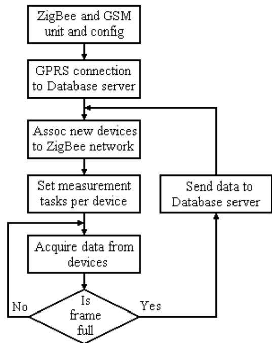
Fig. 4. Operation algorithm of the Coordinator device.
