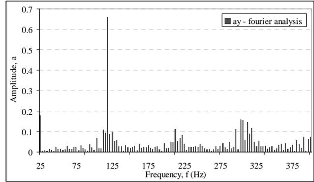
**Fig. 7.** Fourier analysis of  $a_y$  axis from accelerometer data.
