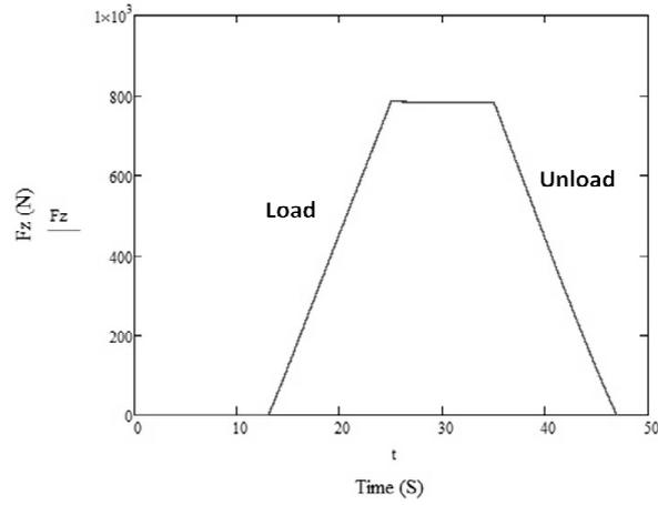
**Fig.8.** Load and unload test for stiffness determination.
