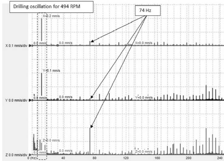
Fig.10. Frequency spectrum on the 494 rpm speed for x, y, and z directions.
