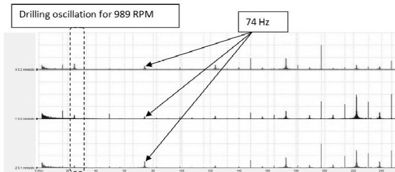
Fig. 11. Dynamic frequency on the 989 rpm speed for x, y, and z directions.
