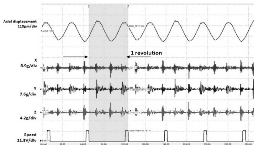
Fig. 12. Vibrations signal during the 989 rpm speed for x, y, and z acceleration and displacement on axial direction.
