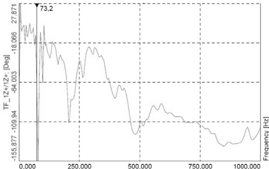
Fig. 5. The frequency response on phase.
