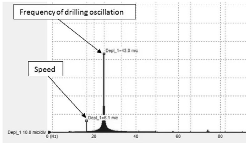
Fig. 13. The axial displacement spectrum for 989 rpm.
