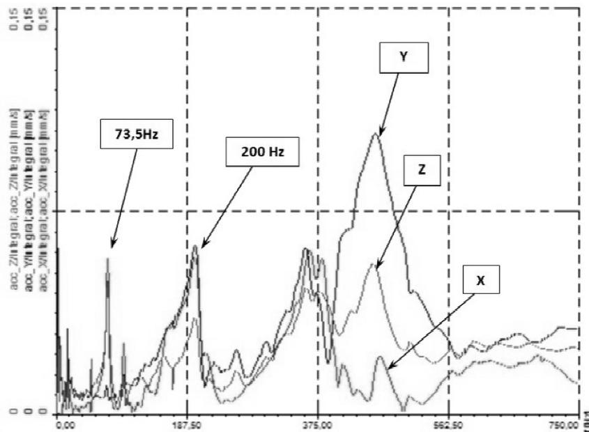
Fig. 7. The frequency spectrum after impact test.
