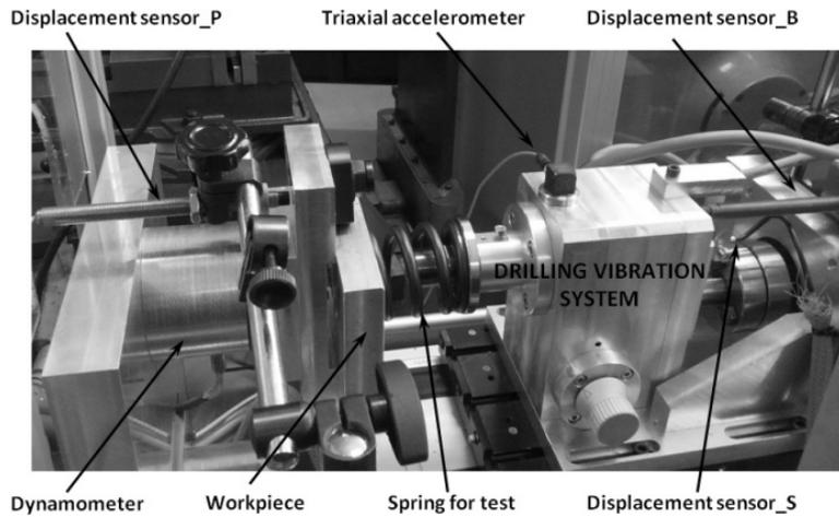
Fig. 2. Experimental setup for static case.
