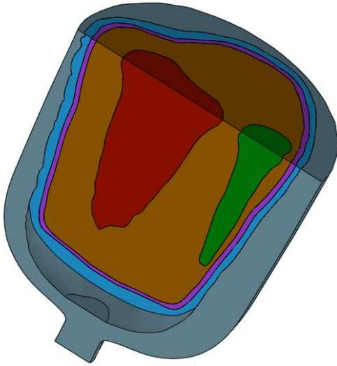
Fig. 4. The assembly cup-stump-liner in section.
