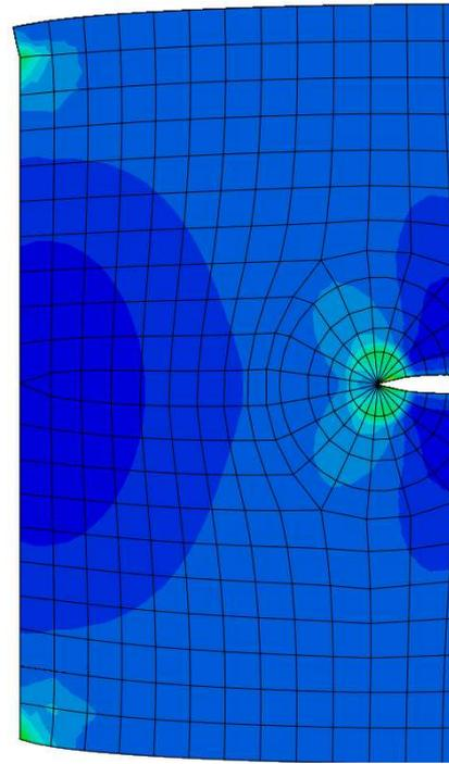
**Fig. 10.** Crack propagation on 2D surface (left half-plane).
