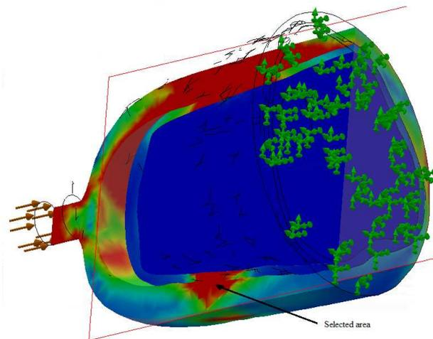
**Fig. 8.** Map of pressure on stump liner interface in section with selected area for crack development.
