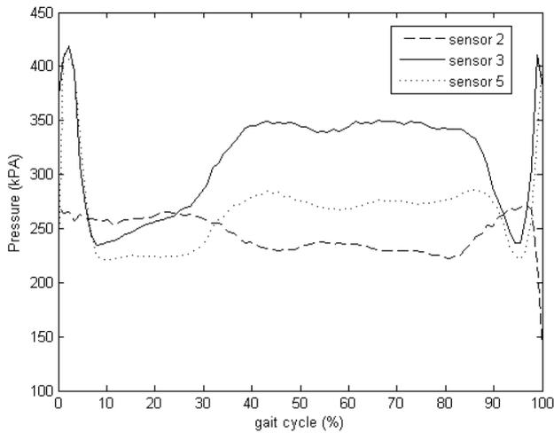
**Fig. 7.** Pressure record by sensor in location 2, 3, and 5 (experimental results).
