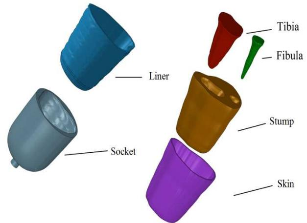
Fig. 3. The parts of modeled assembly stump-liner-socket.
