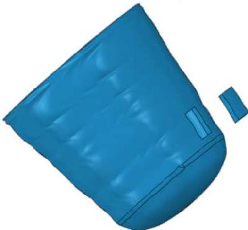
**Fig. 9.** 2D shell used in modeling of crack propagation using cycling loading.
