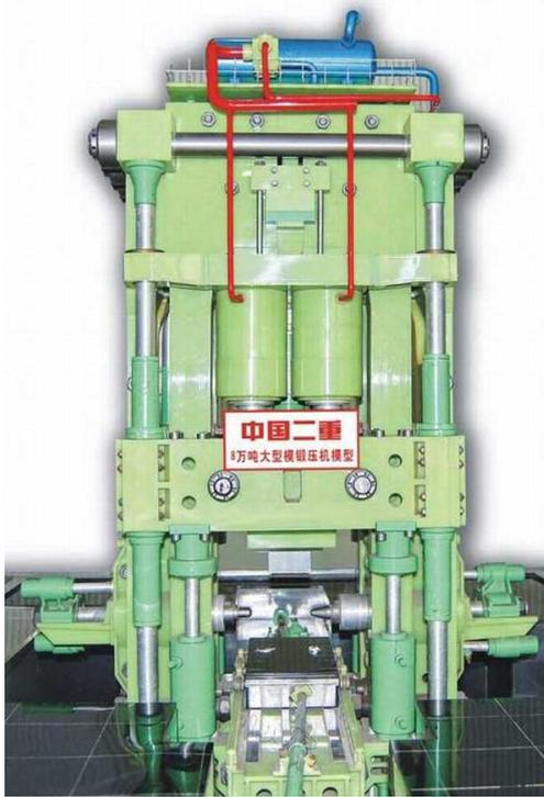
Fig. 3. Example of one-purposed multidirectional forging device – variant 2.
