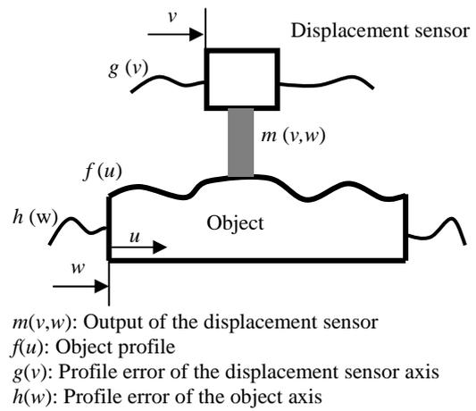
**Fig. 3.** The new method composed of two linear stages.
