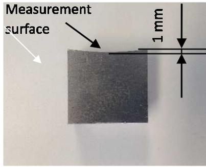
Fig. 6. Measurement object used in the experiment.
