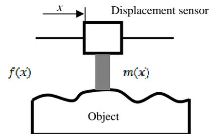
$m(x)$ : Output of the displacement sensor
