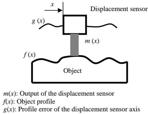
**Fig. 2.** Profile measuring machine consists of displacement sensor and movable mechanism in case of movable mechanism with profile errors.
