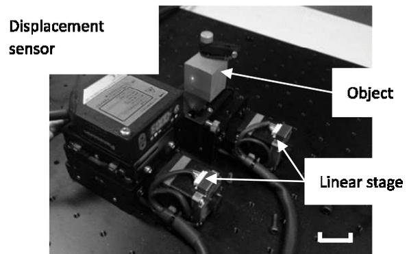
Fig. 5. Experimental equipment to measure the object consists of two linear stages and the displacement sensor.
