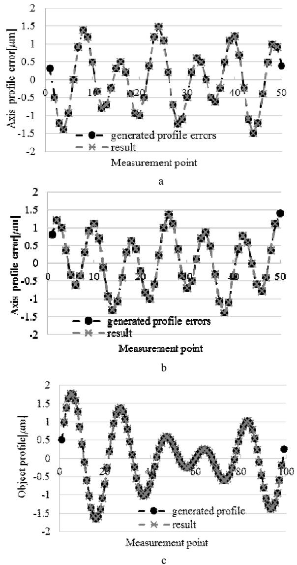
Fig. 4. The generated profile and calculated profile in simulation: a – profile error of the linear stage mounted with the displacement sensor; b – profile error of the linear stage mounted with the object; c – the object profile.
