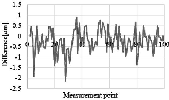
Fig. 8. Difference between the object profile by calculation result and the output of the displacement sensor.
