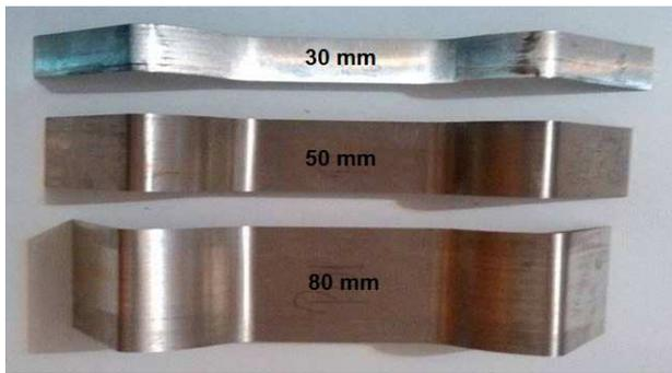
Fig. 9. Influence of width piece on springback.
