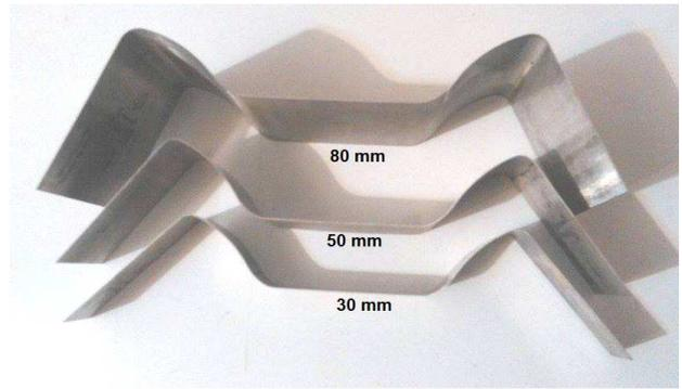
Fig. 7. Influence of forming speed on springback.
