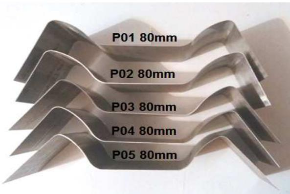
Fig. 6. Influence of the blankholder force on springback.
