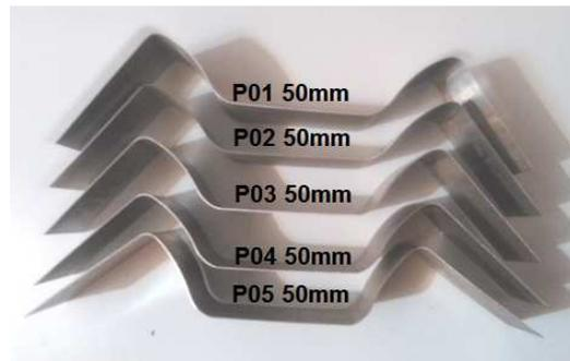
Fig. 5. The influence of the blankholder force on the springback.
