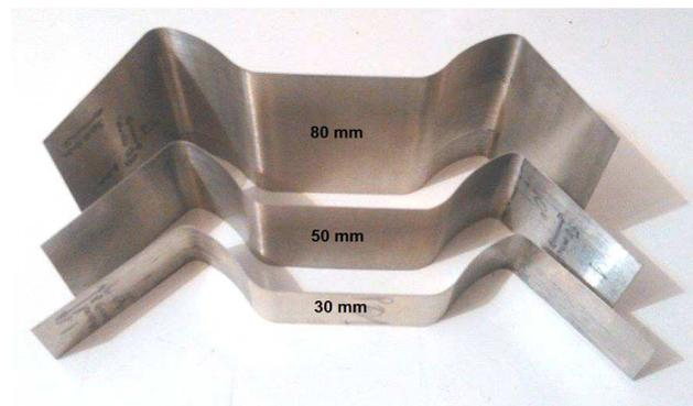
Fig. 8. Influence of rolling direction on springback.
