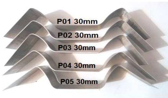
Fig. 4. The influence of the blankholder force on the springback.
