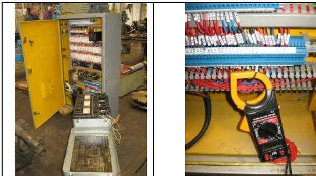
Fig. 6. Measurement of the electrical power consumed by the machine tool.
