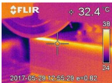
Fig. 7. Cutting temperature measurement using thermal camera FLIR TIP E 45.
