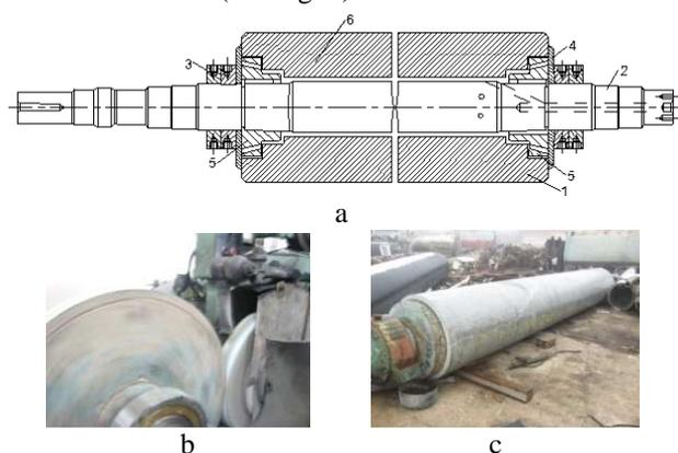
**Fig. 1.** Granite roller: a – cross section (1 – granite cylinder; 2 – shaf; 3 and 4 – tightening washers; 5 – nut; 6 – cement filling; b – granite mantle grinding; c – granite mantle roller.
