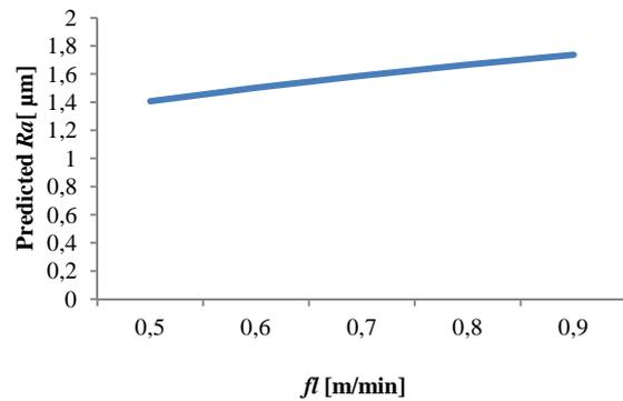
Fig. 13. The longitudinal cutting feed influence over the predicted Ra values.
