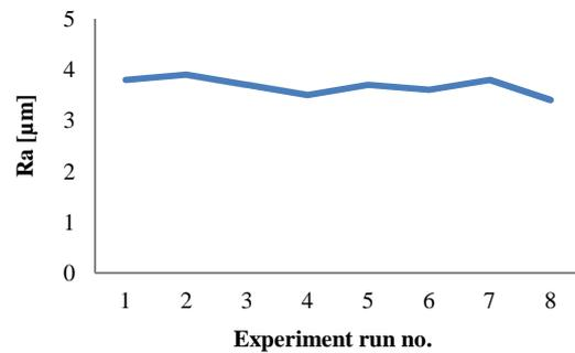
Fig. 9. Surface roughness variation in rough grinding experiments.
