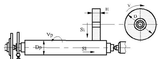
**Fig. 2.** Scheme of external cylindrical grinding process of rollers on special grinding machines tools [2, 3].
