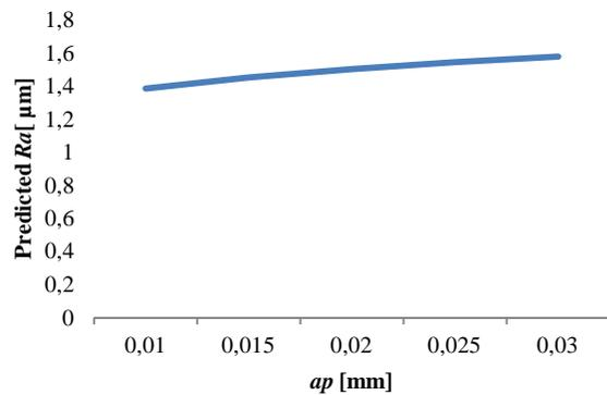
Fig. 14. The cutting depth influence over the predicted Ra values.
