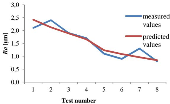
Fig. 11. Measured vs predicted surface roughness values variation in finish grinding experiments.
