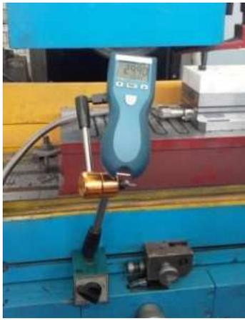
Fig. 5. Grinding disk rotation speed measurement ( $n = 2995$  rpm).
