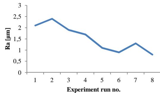
Fig. 10. Surface roughness variation in finish grinding experiments
