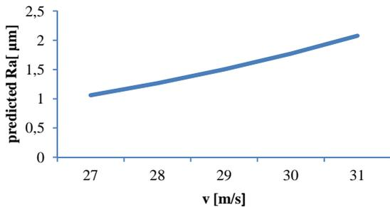
Fig. 12. The cutting speed influence over the predicted Ra values.
