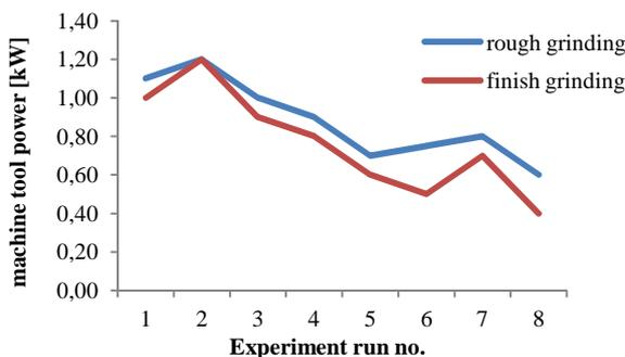
Fig. 8. Machine tool power variation in the rough and finish granite grinding experiments.
