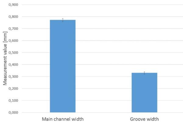
Fig. 10. Measurement results of main channel and grooves.
