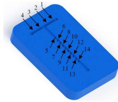
Fig. 9. Measuring positions on micromixer.
