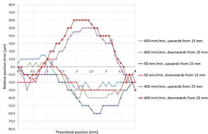
Fig. 4. Positional error at different bed movement velocities.
