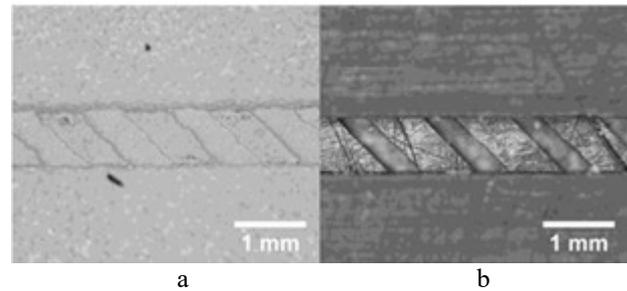
Fig. 11. Digital image of two micromixer channels: *a* – micromixer cast in PDMS [7]; *b* – printed micromixer.
