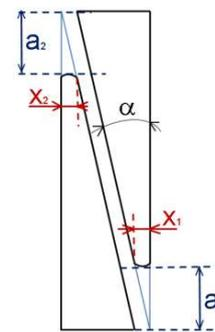
Fig. 6. Dimensions  $x$  are calculated from known angle and measured length  $a$ .
