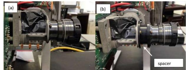
Fig. 2. Mounting of objective to reduce pixel size: a – pixel size is 80 μm without a spacer; b – pixel size is 19 μm with a spacer.
