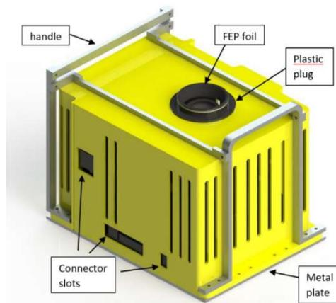
Fig. 3. Custom made casing for optical system.
