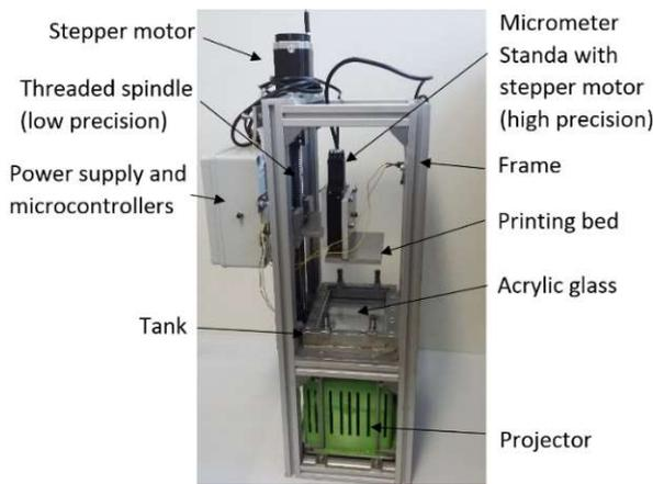
Fig. 1. Custom made stereolithographic DLP printer.
