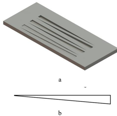
Fig. 5. Test sample to determine printing resolution: a – model of the test piece; b – the ground plan of the channels.
