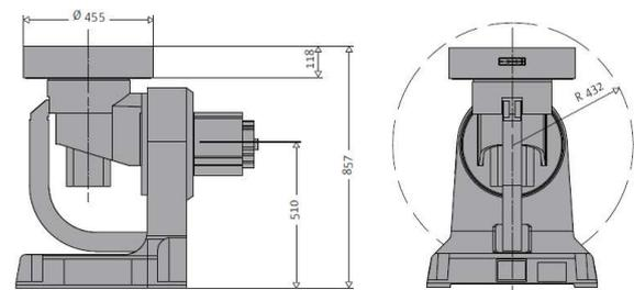
Fig. 7. Overall dimensions and workspace DKP-400, two-axis positioning unit [10].
