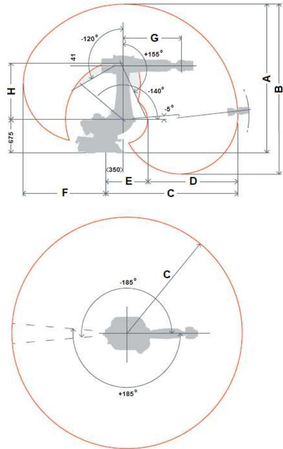
Fig. 6. Overall dimensions and workspace of KR 210 R2700 extra industrial robot [10].
