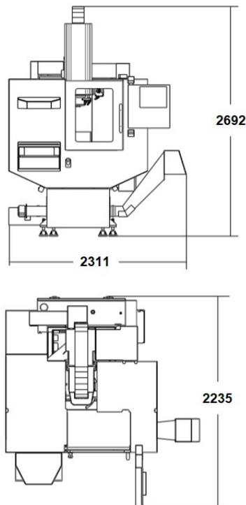
Fig. 5. Overall dimensions of Haas Mini Mill CNC machine-tool [9].
