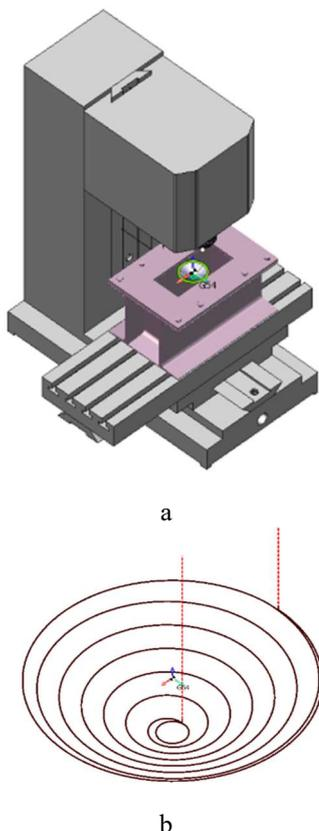
**Fig. 9.** Strategy 1: *a* – kinematic model of Haas Mini Mill CNC machine-tool; *b* – spiral processing toolpath.
