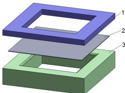
Fig. 2. Forming tool system.
