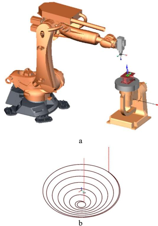
**Fig. 10.** Strategy 2: *a* – kinematic model Kuka KR 210 R2700 extra industrial robot; *b* – spiral processing toolpath.
