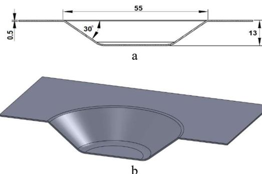
Fig. 8. The processed part: a – dimensions; b – 3D model.
