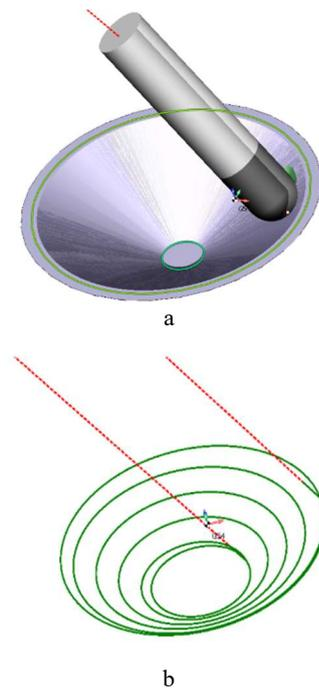
**Fig. 11.** Strategy 3: *a* – tool perpendicular on the part walls; *b* – spiral processing toolpath.
