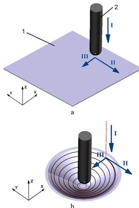
Fig. 1. Incremental forming: a – workpiece; b – part.
