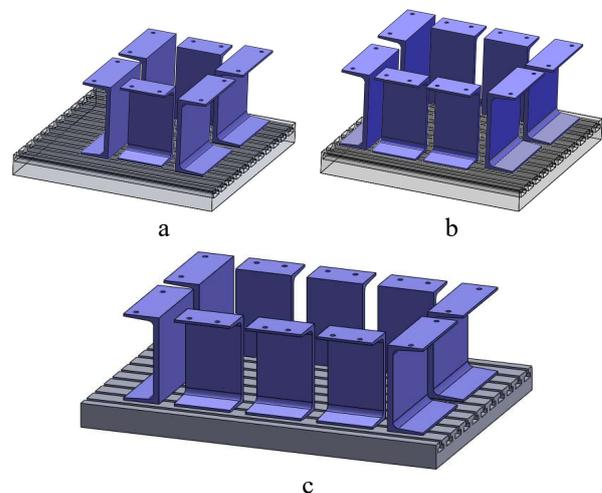
Fig. 4. Modular active plates: a – 6 U-profiles; b – 8 U-profiles; c – 6 U-profiles.
