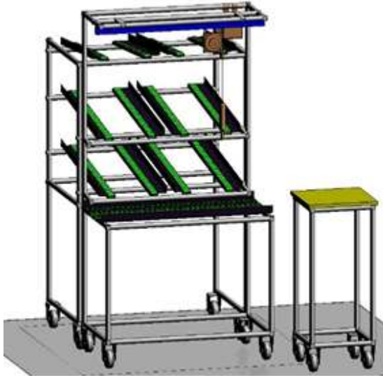
Fig. 5. The 3D model of a modular-flexible workstation.
