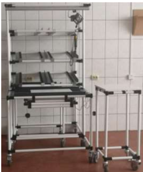
Fig. 7. The photo of a modular-flexible workstation.
