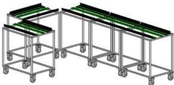
Fig. 6. The 3D model of a modular-flexible transport system.
