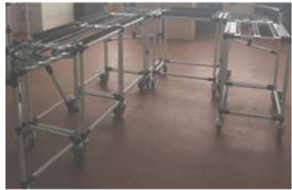
Fig. 8. The photo of the modular-flexible transport system.
