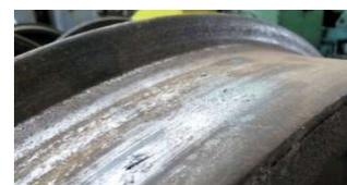
Fig. 3. Example of worn wheel running surface.
