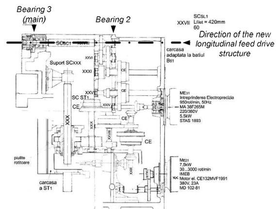
Fig. 6. Conventional structure and new feed drive axis.
