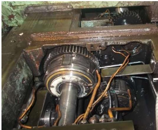
Fig. 8. Longitudinal lead screw – gears and rear radial bearing.
