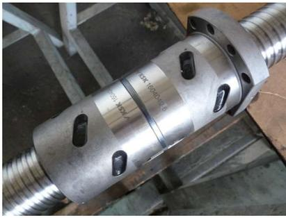
Fig. 13. Ball screw and nut detail.
