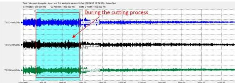
Fig. 29. The vibration waveform during the cutting process after modernization.
