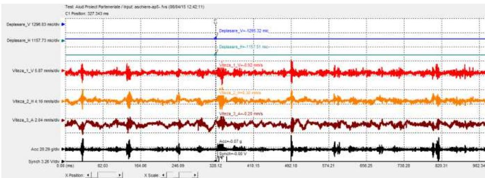
Fig. 28. The vibration waveform during the cutting process before modernization.
