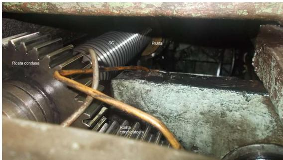
Fig.7. Longitudinal lead screw – gears and thread.
