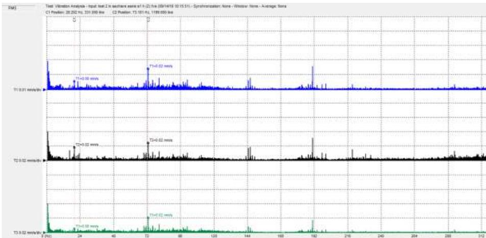
Fig. 26. Frequency spectrum on Z direction – carriage no. 1 during the cutting process.
