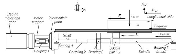
Fig. 4. The kinematic structure of the longitudinal feed drive.
