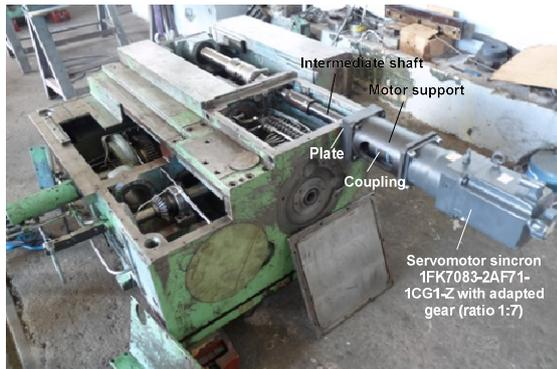
Fig. 14. View of the refabricated longitudinal axis.
