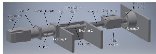
Fig. 5. The 3D model of the longitudinal feed drive.
