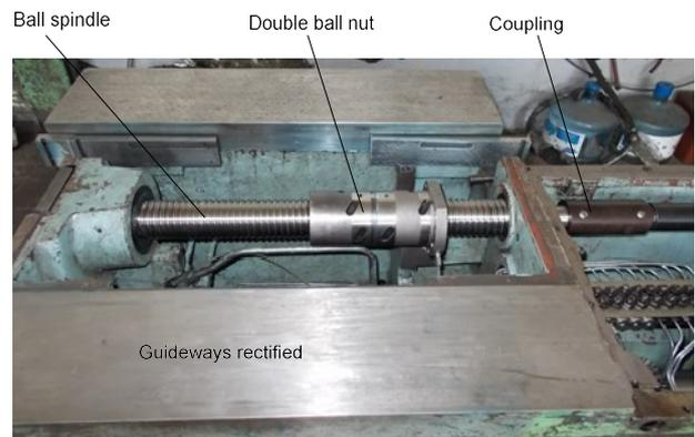
Fig. 12. New longitudinal feed drive – ball screw and nut mounted.
