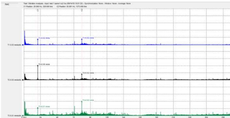
Fig. 27. Frequency spectrum on Z direction – carriage no. 2 during the cutting process.
