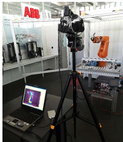
Fig. 5. Experimental setup for ABB IRB 120 robot thermal behavior analysis.
