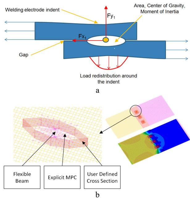
**Fig. 4.** The proposed approach: *a* – schematic representation; *b* – FEM model and normal stress distribution.
