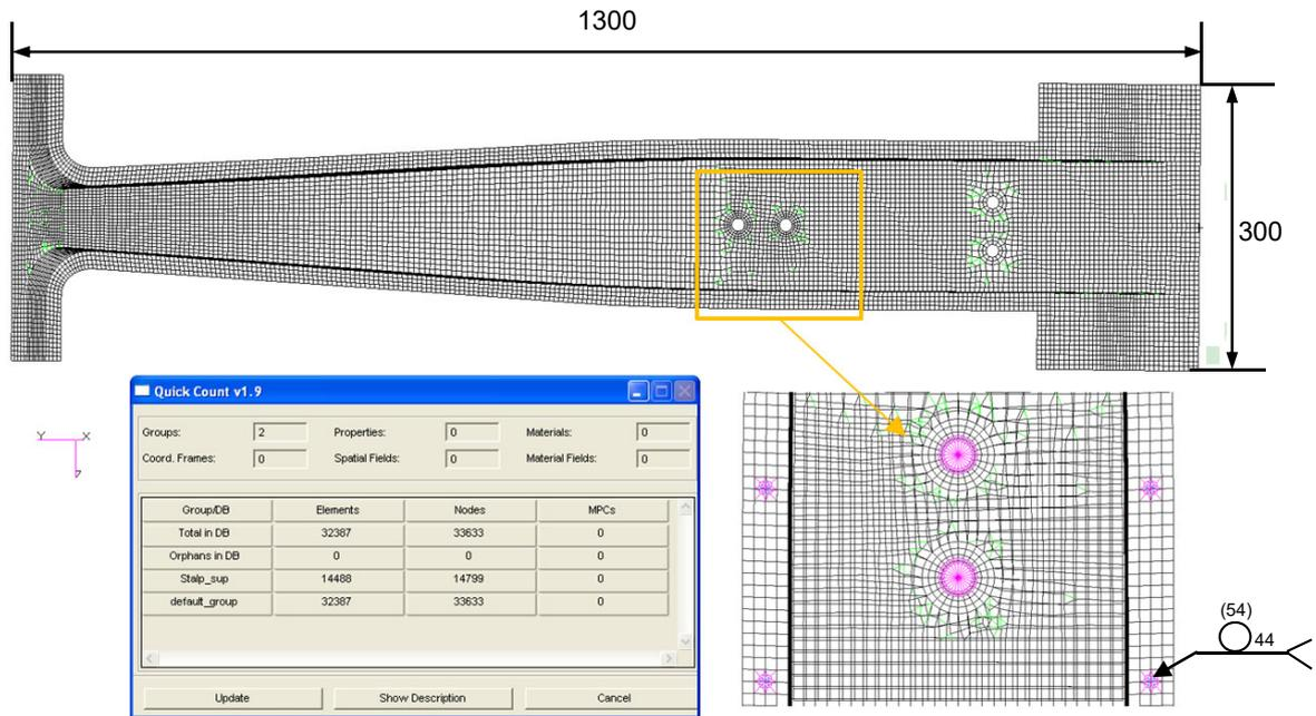
Fig. 6. Details regarding the geometry, mesh, number of elements and nodes, as well as the definition of spot welds and shear bolts.
