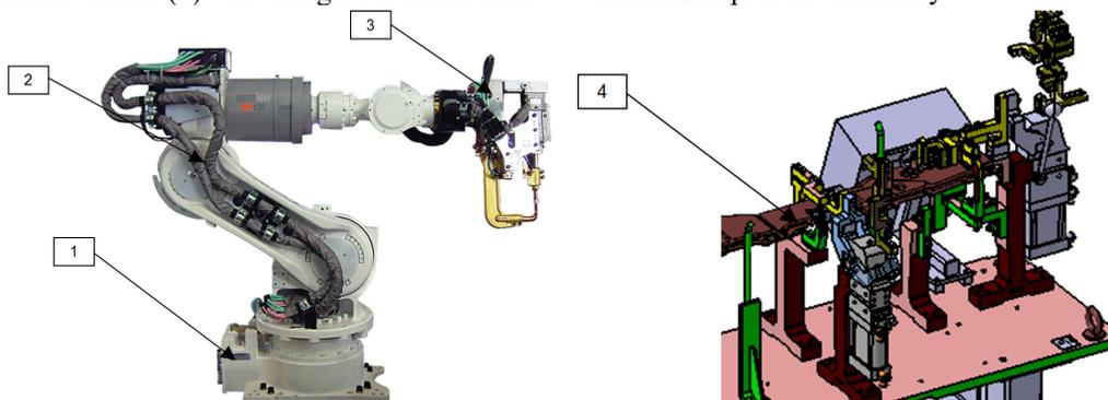
Fig. 1. Typical setup of a spot welding cell: 1 – industrial robot, 2 – cable dressing, 3 – spot welding end-effector, 4 – semi or fully automated welding fixture.
