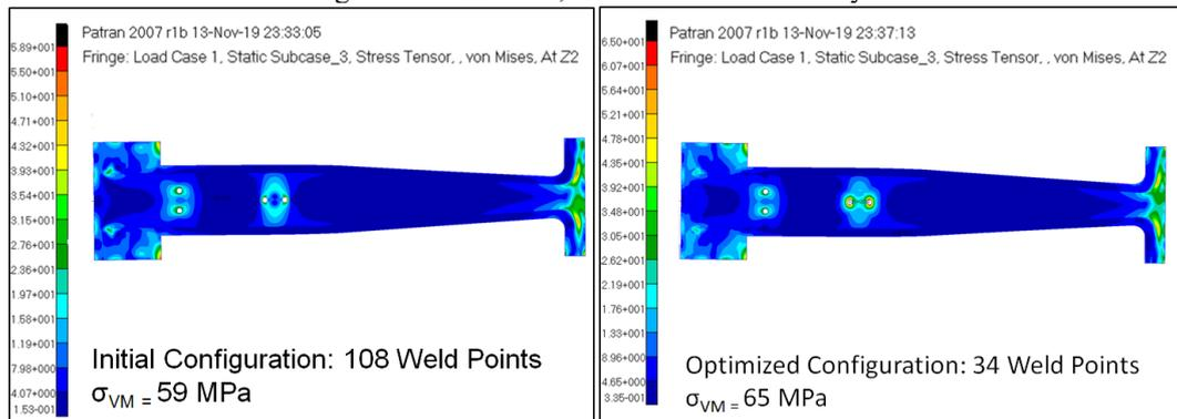
Fig. 7. Equivalent Von Mises stress for the initial and the updated configurations.
