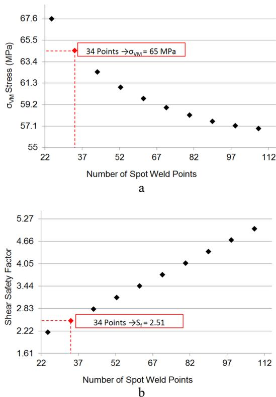
Fig. 8. Relationship between the number of spot weld points and: a – equivalent Von Mises stress (MPa); b – shear safety factor.
