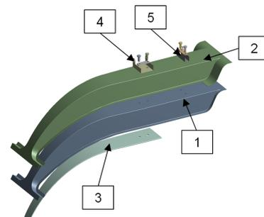
**Fig. 5.** Assembly of the car B-pillar: 1 and 2 – interior and exterior sheet metal bodies, 3 – reinforcing plate, 4 and 5 – hinge supports.
