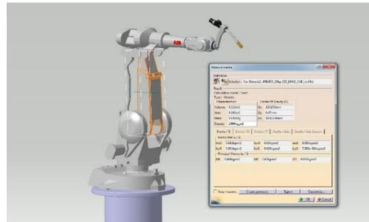
**Fig. 15.** Identifying the partial volume and mass center coordinates of IR partial assembly corresponding to the mobile part of IR joint 2 and fixed part of joint 3 [3, 10].
