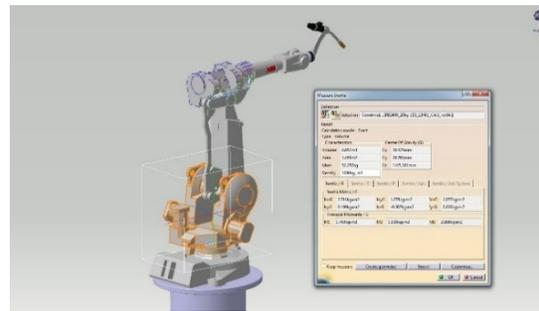
**Fig. 14.** Identifying the partial volume and mass center coordinates of IR partial assembly corresponding to the mobile part of IR joint 1 and fixed part of joint 2 [3, 10].
