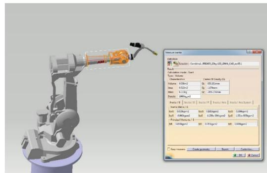
**Fig. 17.** Identifying the partial volume and mass center coordinates of IR partial assembly corresponding to the mobile part of IR joint 4 and fixed part of joint 5 [3, 10].
