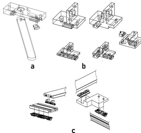
**Fig. 4.** Component details: a – rotating panel stop sub-assembly; b – custom bases for stepper motors, bearing blocks, limit switches; c – POM sliders between extruded profiles.
