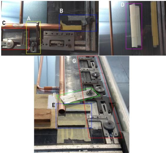
**Fig. 2.** Manual fixturing components (A – header hook locator, B & E – a header block locator supported by a fastened support element, C & G – one row of evenly spaced panel locators, D – a panel side's thin block locator affixed with adhesive tape, F – a custom pivot hold down clamp).
