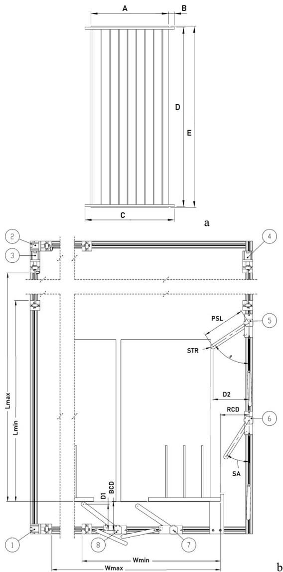
**Fig. 5.** a – Typical product dimensions needed to configure the fixture (A – panel width, B – header exit length, C – grid width, D – grid length, E – panel length); b – required geometrical properties of the fixture (motors numbered 1 to 8).
