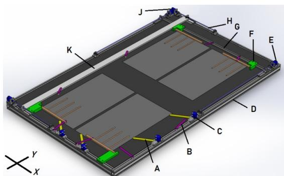
**Fig. 3.** Designed fixture (solar absorber is only partly shown for simplicity); A – panel locator, B – pivot hold-down clamp, C – panel locator motor, D – frame, E&J – cartesian mechanism motor, F – corner locator, G – cartesian mechanism X bar, H – lead screw mechanism for K, K – cartesian mechanism Y bar).
