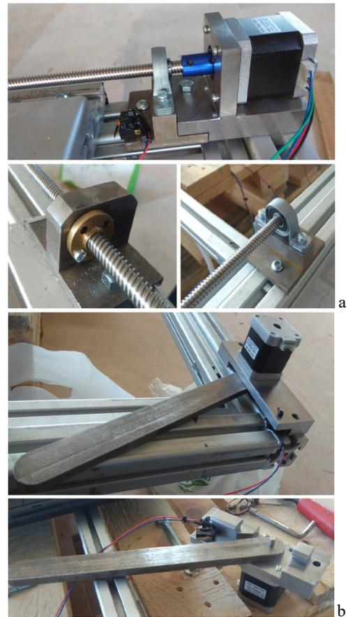
Fig. 7. Assembled components: a – the left end of the bar; b – the rotating panel locator.
