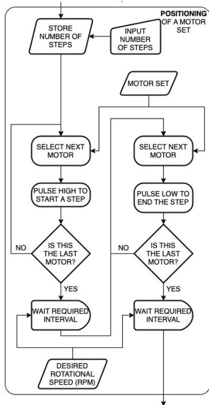
Fig. 6. Flowchart of the microcontroller program used during testing.
