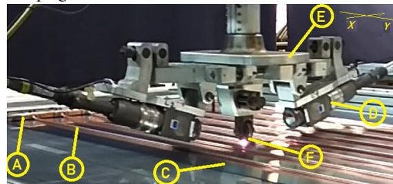
**Fig. 1.** Laser station (A – header tube, B – riser tube, C – thin sheet panel, D – laser head, E – gantry carriage, F – laser carriage wheel).
