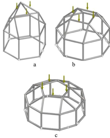
**Fig. 5.** FEA boundary condition: *a* – elongated triangular cupola; *b* – elongated square cupola; *c* – elongated pentagonal cupola.
