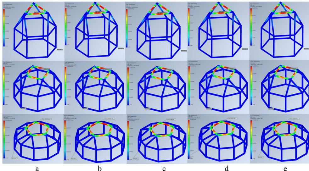
**Fig. 9.** FEA displacement results for aluminium 6061 material assigned: *a* – 500 N load applied; *b* – 1000 N load applied; *c* – 2000 N load applied; *d* – 3000 N load applied; *e* – 4000 N load applied.
