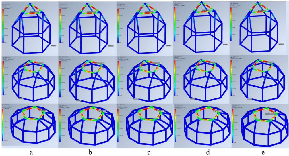
**Fig. 8.** FEA displacement results for stainless-steel material assigned: *a* – 500 N load applied; *b* – 1000 N load applied; *c* – 2000 N load applied; *d* – 3000 N load applied; *e* – 4000 N load applied.
