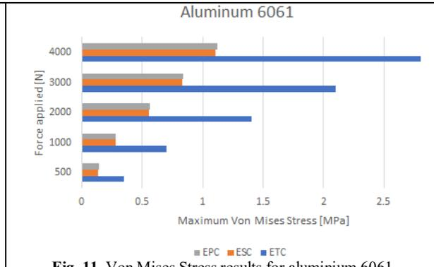
Fig. 11. Von Mises Stress results for aluminium 6061.
