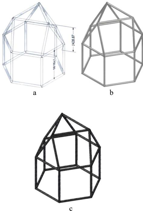
**Fig. 2.** Elongated triangular cupola: *a* – approximated dimensions of elongated triangular cupola structure; *b* – material applied to elongated triangular cupola structure; *c* – 3D model mesh.
