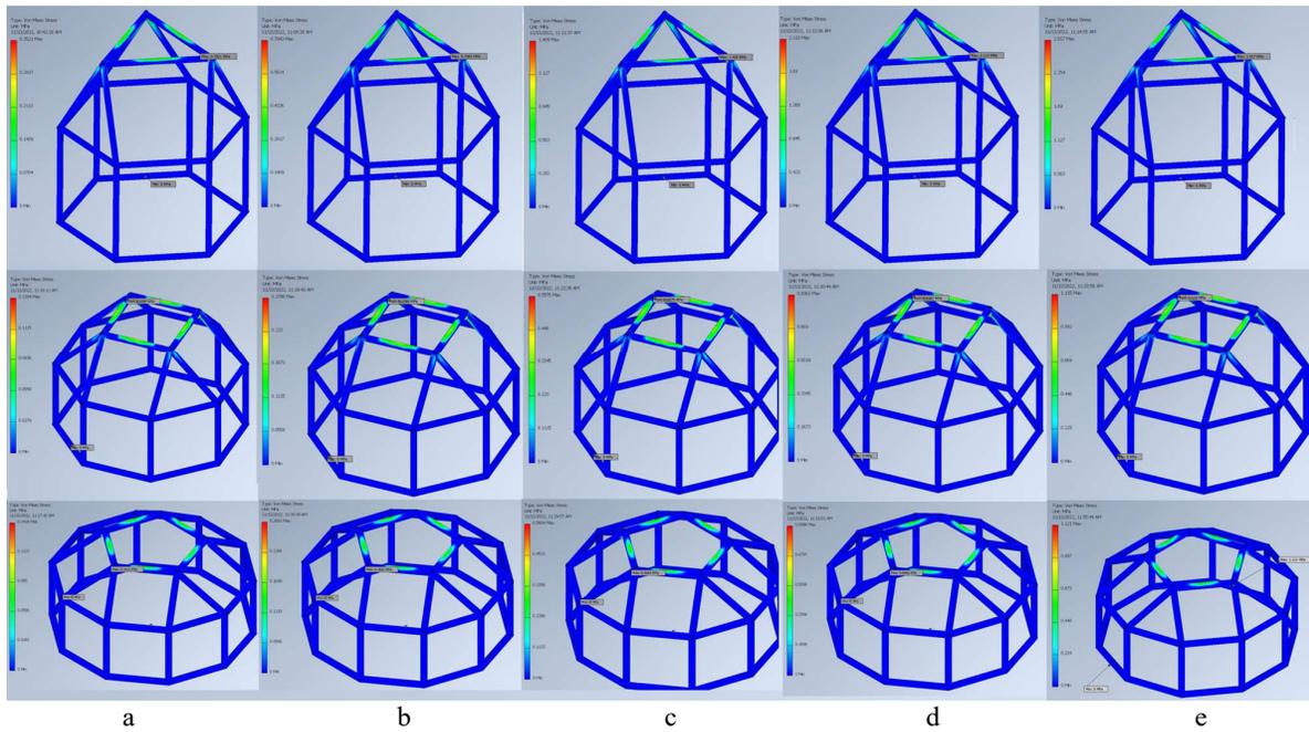
Fig. 6. FEA Von Mises Stress results for stainless-steel material assigned: a – 500 N load applied; b – 1000 N load applied; c – 2000 N load applied; d – 3000 N load applied; e – 4000 N load applied.
