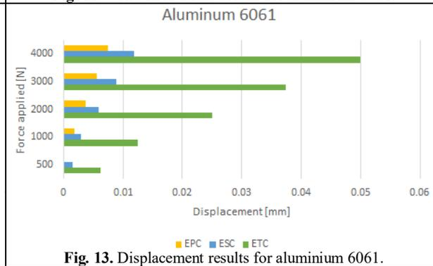
Fig. 13. Displacement results for aluminium 6061.
