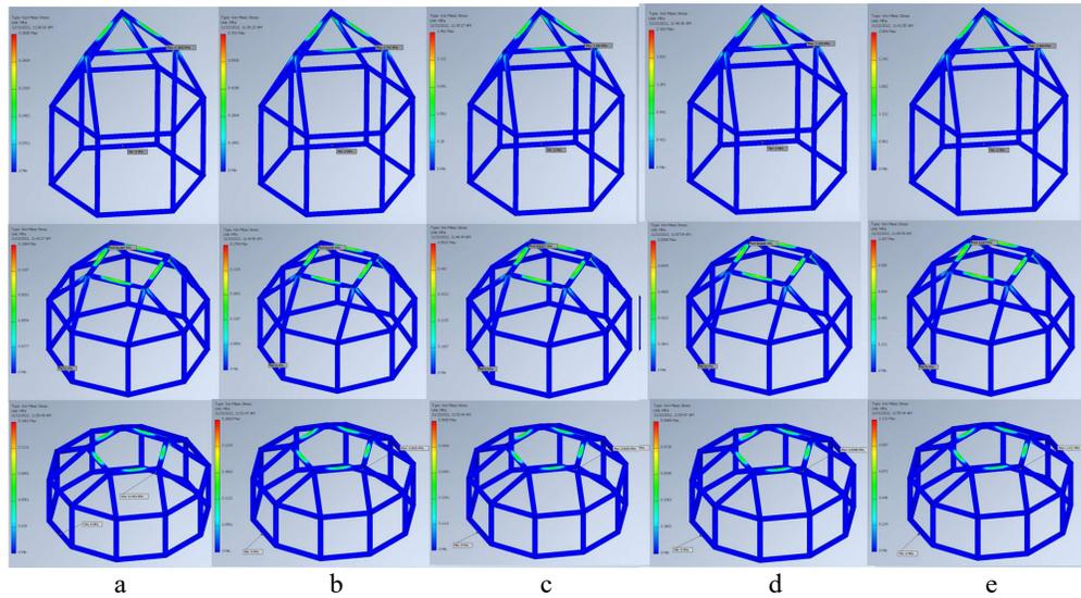
**Fig. 7.** FEA Von Mises Stress results for aluminium 6061 material assigned: *a* – 500 N load applied; *b* – 1000 N load applied; *c* – 2000 N load applied; *d* – 3000 N load applied; *e* – 4000 N load applied.
