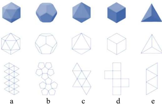
**Fig. 1.** Platonic polyhedra: *a* – icosahedron; *b* – dodecahedron; *c* – octahedron; *d* – cube; *e* – tetrahedron.
