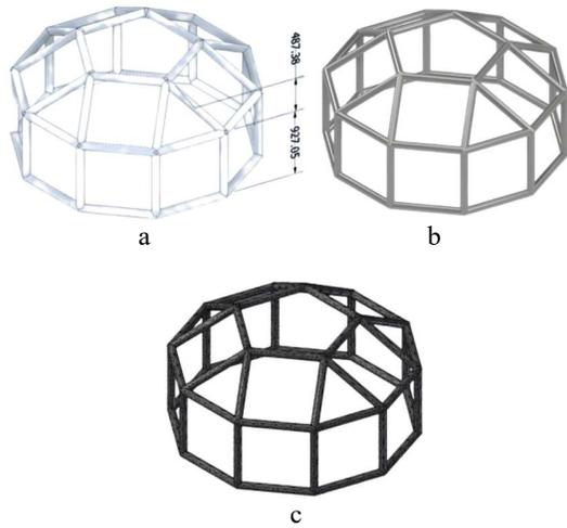
**Fig. 4.** Elongated pentagonal cupola: *a* – approximated dimensions of elongated pentagonal cupola structure; *b* – material applied to elongated pentagonal cupola structure; *c* – 3D model mesh.
