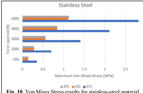
Fig. 10. Von Mises Stress results for stainless-steel material.
