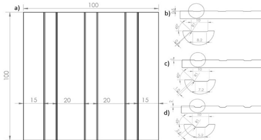
**Fig. 1.** Technical drawings for: a – channel positioning on stainless steel plate 304; b – channel with a depth of 0.5 mm; c – 1 mm; d – 2 mm.
