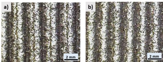
Fig. 5. Optical micrographs of the deposited material with an overlap of: a – 32%; b – 47%.
