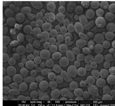
**Fig. 3.** SEM micrographs of the SS304 powder used in the experiments.
