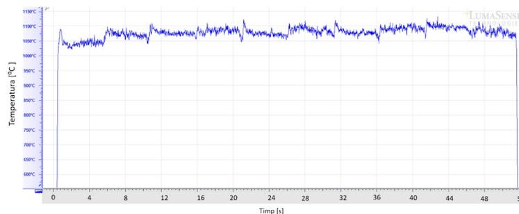
**Fig. 9.** Temperature fluctuations during the LMD process.
