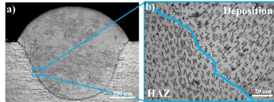
Fig. 7. Optical micrographs of the microstructure of deposited SS304 (a) and a zoom in the interface zone (b) showing δ-ferrite dendrites in the austenite matrix.
