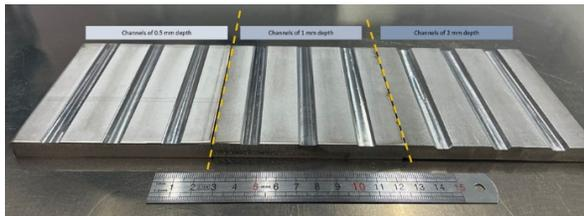
**Fig. 2.** Channels with different depths obtained by a subtractive process.
