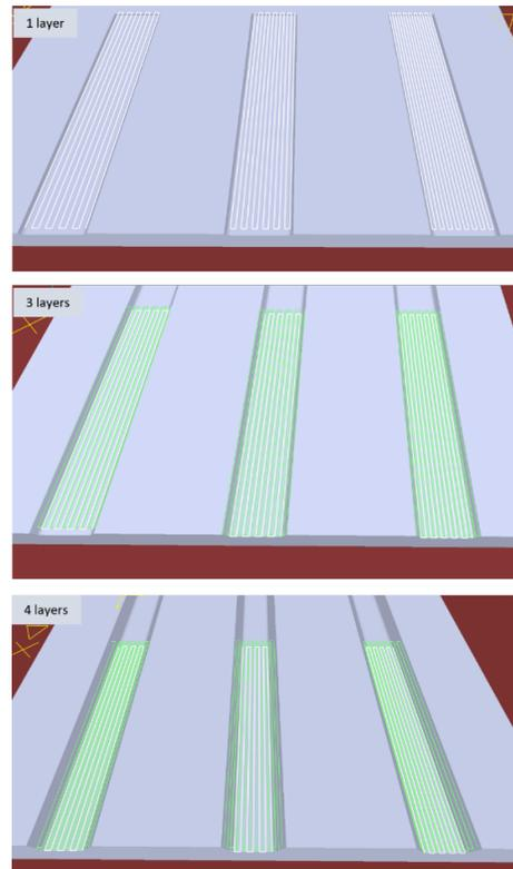
Fig. 4. Scanning strategy used for repairing process by covering channels with different depths obtained by a subtractive processing method.
