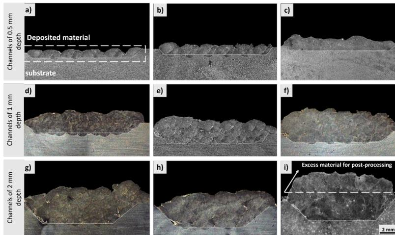
**Fig. 8.** Cross-section images of the channels rectified by coating using the LMD technique with depths of: a-c – 0.5 mm; d-f – 1 mm; g-i – 2 mm.
