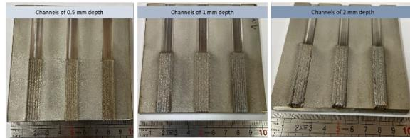
Fig. 6. Rectification by coating using the LMD technique of channels with different depths.
