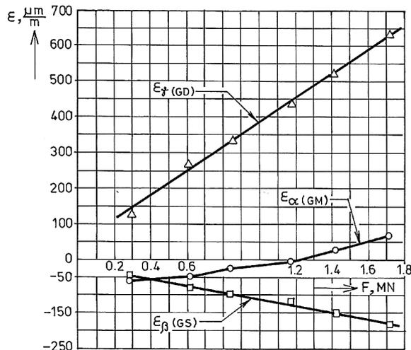
Fig. 4. Gauging diagram for rosette G in the state "WP", the third experiment.
