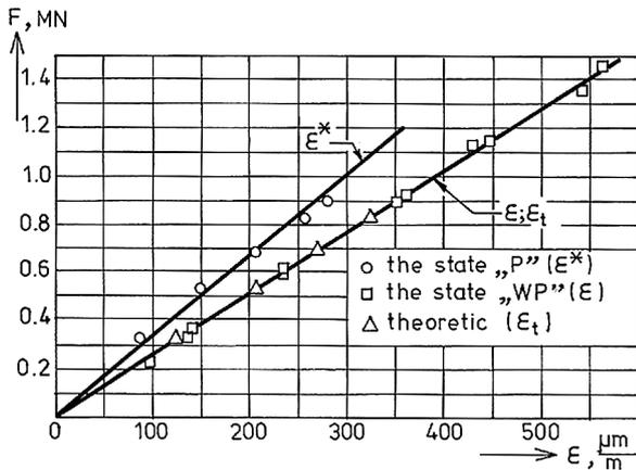
Fig. 3. Gauging diagrams of the captor F1.
