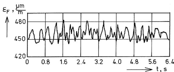
Fig. 6. Variation of deformation of the drill pipe body due to the tensile force ( $\epsilon_F$ ) for  $W_B = 120 \text{ kN}$  and  $n_B \approx 10 \text{ rot/min}$ .
