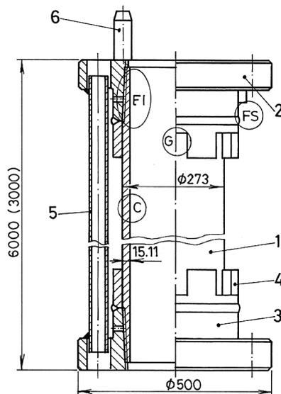
**Fig. 1.** Drilling pipe with air tubes: 1– body; 2 – upper flange; 3 – lower flange; 4 – collar with crenels; 5 – air tube; 6 – centre bolt.
