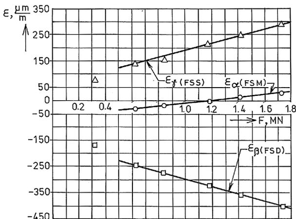
Fig. 5. Gauging diagram for rosette FS in the state "WP", the third experiment.
