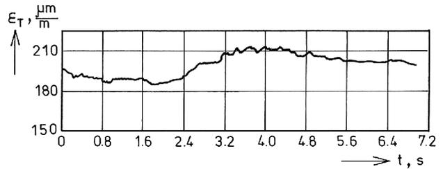
Fig. 7. Variation of deformation of the drill pipe body due to the torsion moment ( $\epsilon_T$ ) for  $W_B = 200 \text{ kN}$  and  $n_B \approx 10 \text{ rot/min}$ .
