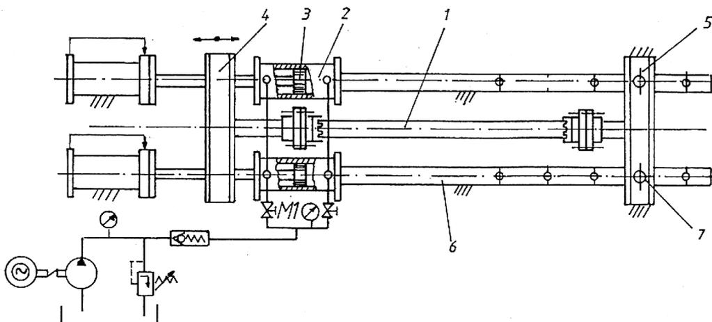
Fig. 2. Scheme of the working stand used for tensile loading of captors: 1 – loading captor; 2 – hydraulic cylinder; 3 – piston; 4 – mobile traverse; 5 – fixed traverse; 6 – guiding elements of the fixed traverse; 7 – fixing bolt.
