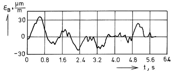
Fig. 8. Variation of deformation of the drill pipe body due to the bending moment ( $\epsilon_B$ ) for  $W_B = 140 \text{ kN}$  and  $n_B \approx 10 \text{ rot/min}$ .
