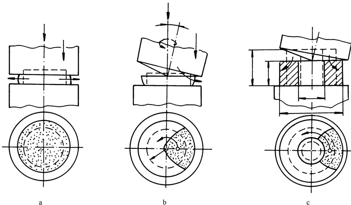
Fig. 2. Material flowing during volumetric forming: a – conventional pressing of cylindrical pieces; b – full cylindrical pieces cold forming by using an oscillatory die; c – cylindrical ring type pieces cold forming by using an oscillatory die.
