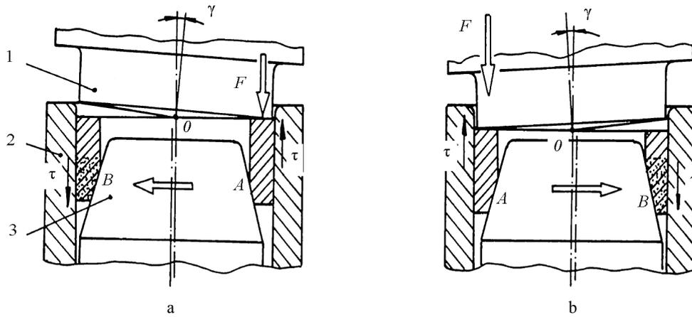
Fig. 4. Material flowing mechanism during volumetric pressing of tapered rings by using an oscillatory die: a – central punch, 3, oscillates to the left; b – idem, to the right.
