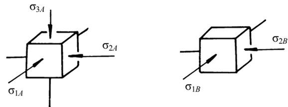
Fig. 5. Stresses conditions in zones A and B.
