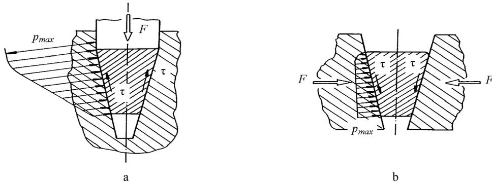
Fig. 3. Wedge type pieces manufacturing by forming: a – direct extrusion; b – cyclic flattening.
