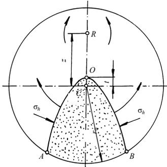
**Fig. 6.** Material flowing mechanism during orbital volumetric forming.
