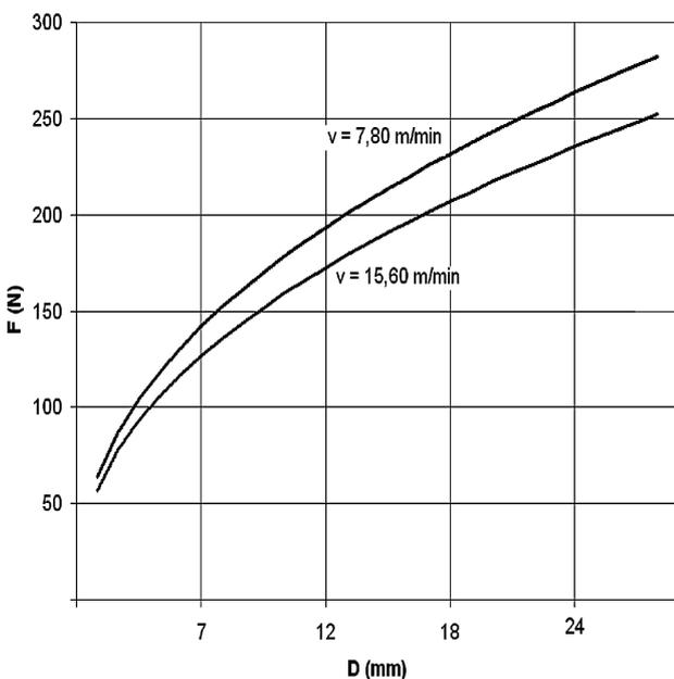
Fig. 5. The variation of axial force as a function of drill diameter, for different drilling feed rates.
