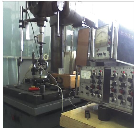
Fig. 1. The image of the stand of determinations with the force moment pickup and the registration system.
