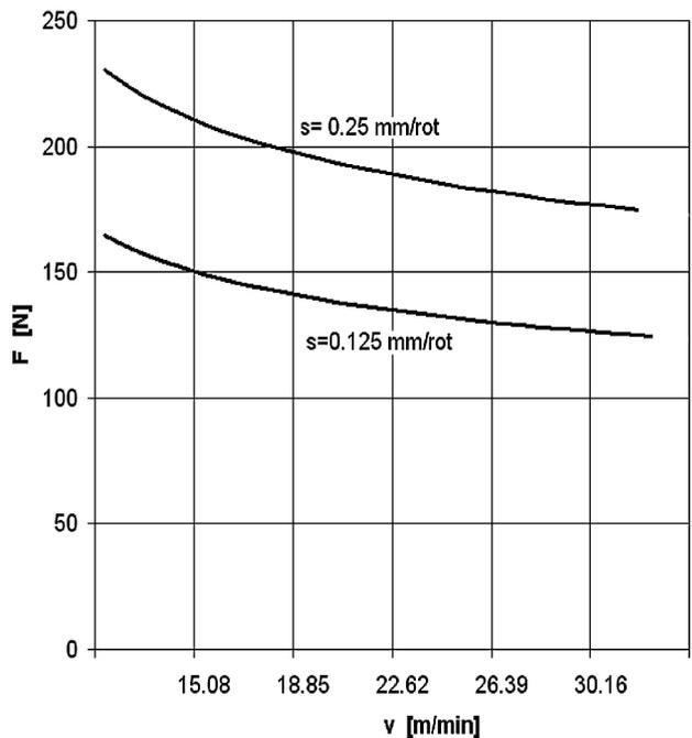
Fig. 7. The variation of axial force as a function of drilling speed, for different feed rates.
