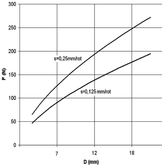
Fig. 4. The variation of axial force as a function of drill diameter, for different feed rates.
