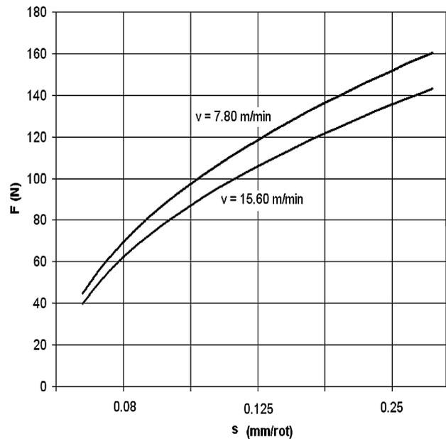
Fig. 3. The variation of the axial force as a function of feed rate, for different drilling speeds of the tool.
