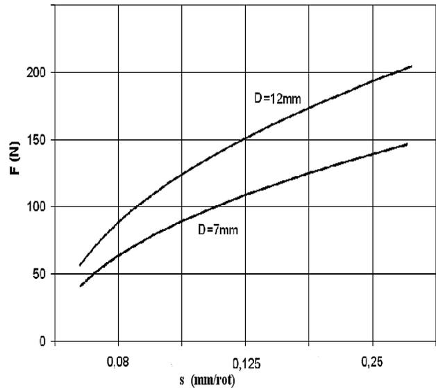
Fig. 2. The variation of the axial force of feed rate, for different drill diameters.
