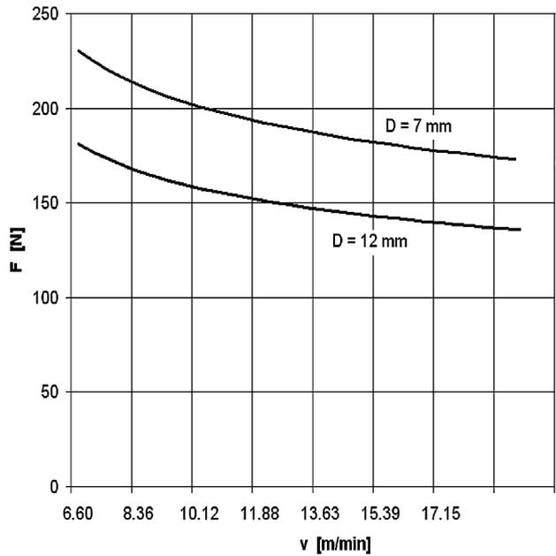
Fig. 6. The variation of axial force as a function of drilling speed, for different hole diameters.
