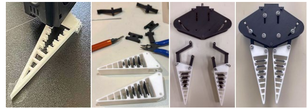
Fig. 9. Prototype manufacturing phases (left to right): frame 3D printing, finger assembly, linkage assembly, assembled gripper.
