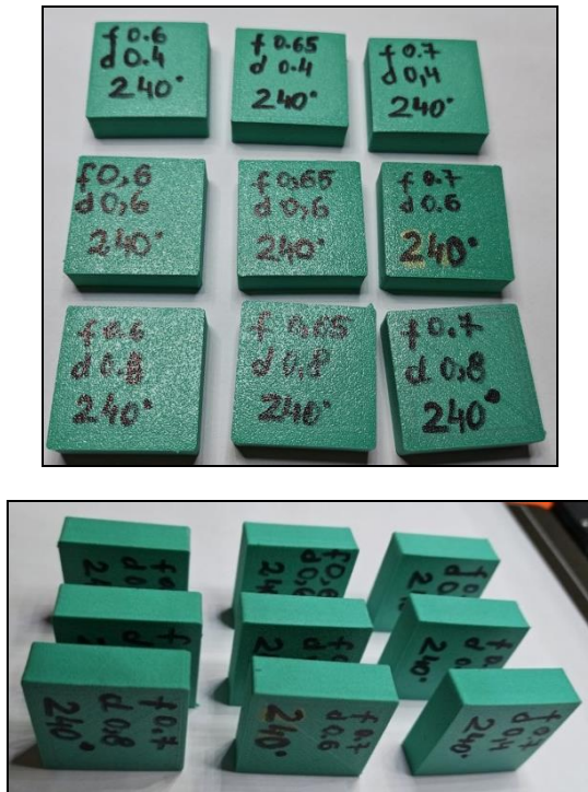
Fig.2. varioShore samples, 3D-printed in different parameters' configurations.
