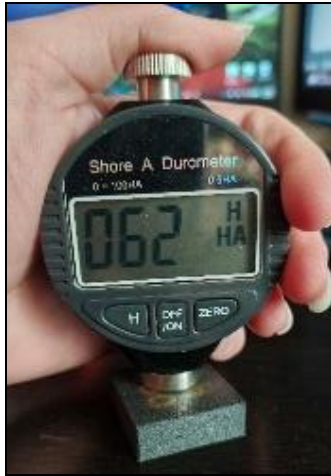
Fig. 4. Shore A hardness measurement of the printed samples (230 °C, 0.8 flow rate factor).
