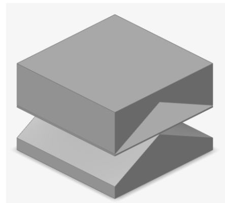
Fig. 4. The 3D model of the die, punch, and sheet metal blank.
