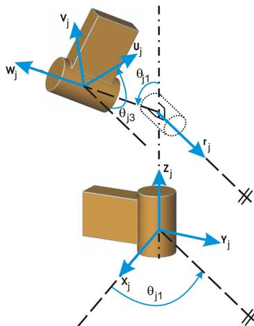
Fig. 9. Spherical joint.
