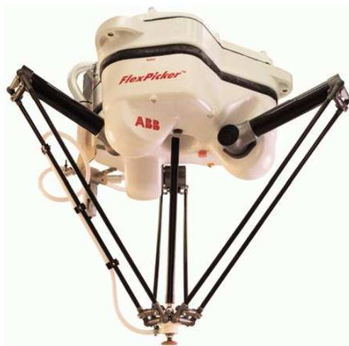
Fig. 1. Delta parallel robot.
