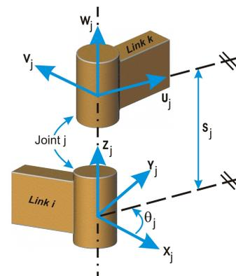
Fig. 7. Revolute, prismatic and cylindrical joints.
