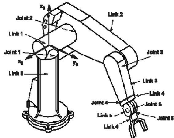
Fig. 2. Vertical knick arm robot.
