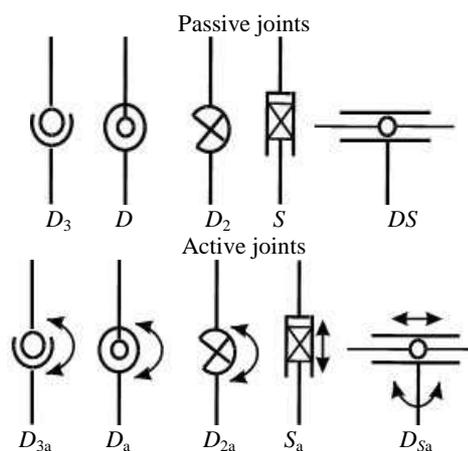
Fig. 5. Main different types of joints used in parallel robots.
