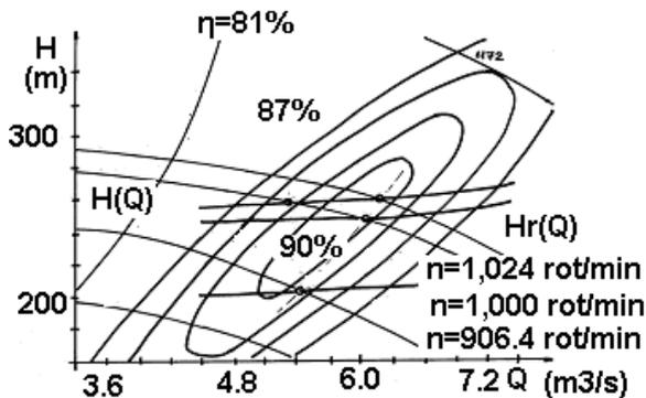
Fig. 1. A sequence of the characteristics curves of the two centrifugal pumps in parallel.
