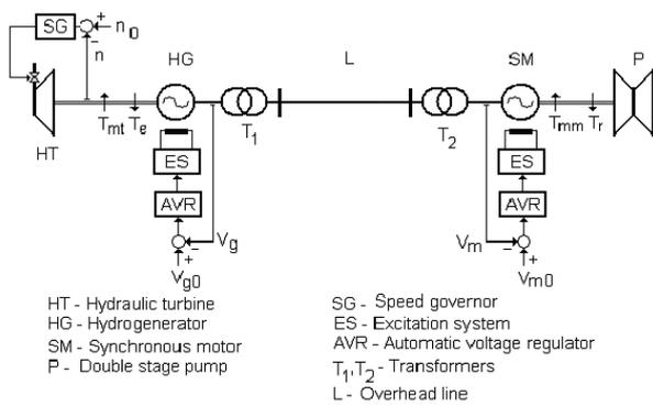
Fig. 3. The power electric simulated system.
