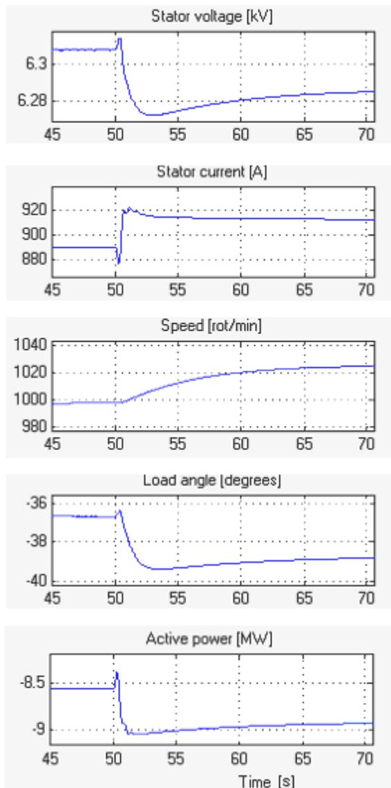
Fig. 5. Synchronous motor transients.
