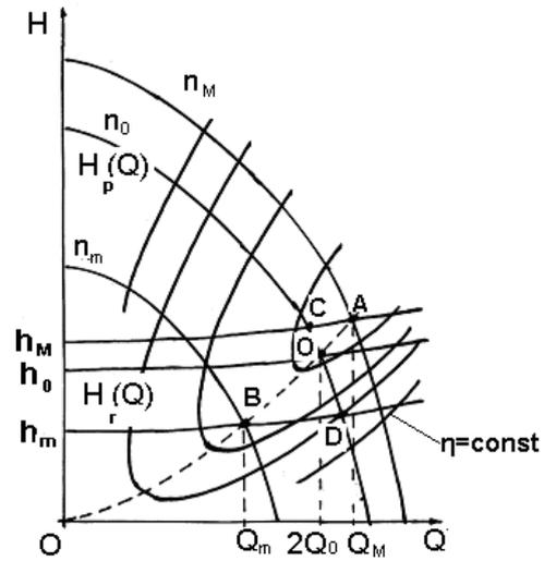
Fig. 2. Explanatory plotting head-capacity-speed-efficiency of the pumps with network.
