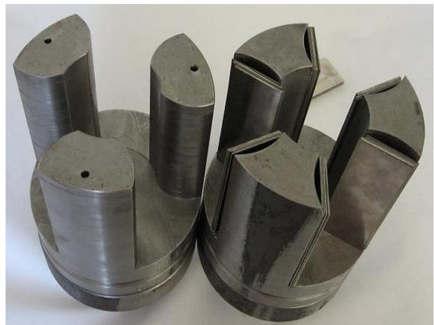
Fig. 1. Elastic coupling with dumping SERB-CEL 130.
