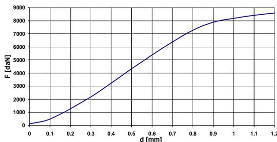
Fig. 3. The inflection characteristic for 3 stratified lamellas of 2 mm thickness.
