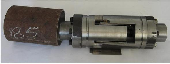
Fig. 2. Elastic coupling with assembled dumping SERB-CEL 130.
