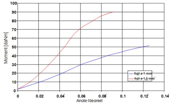
Fig. 5. Moment – angle characteristic for different lamella sets thickness.
