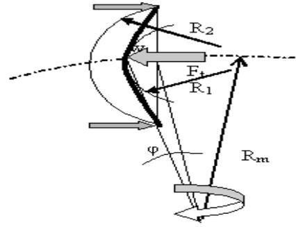
Fig.6. The dimensions defining for the torsion moment calculation.
