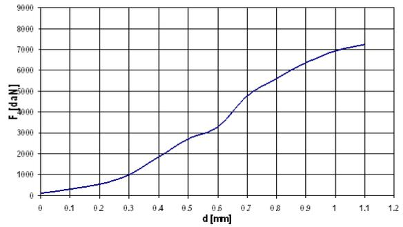
Fig.4. The inflection characteristic for one stratified lamella of 2 mm thickness.
