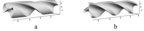
**Fig. 2.** Body of a drill with two grooves (a) and three grooves (b).
