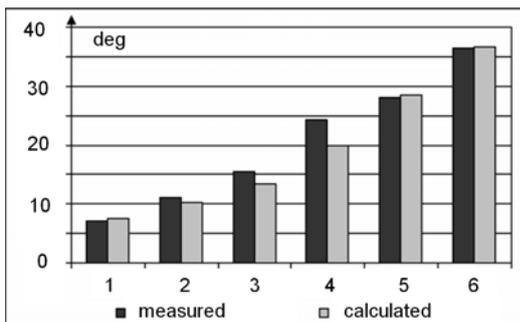
Fig. 8. Comparison of experimental and theoretical results for primary shear angle.
