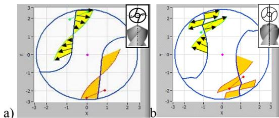
Fig. 12. Radial force repartition for: a) standard drill, b) step drill.
