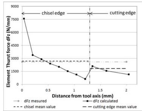
Fig. 9. Example of thrust force results for drilling tests for the central element.
