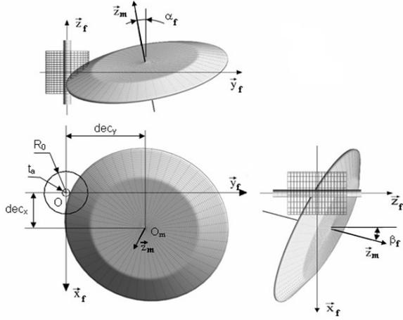
**Fig. 1.** Position definition of the finishing grinding wheel in the reference mark related to the drill.
