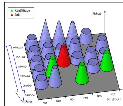
Fig. 14. Evolutions of the parameter Hdcol according to the tool wear.
