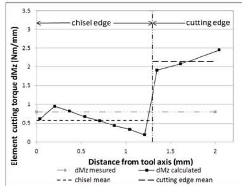
Fig. 10. Example of Cutting torque results for drilling tests for the central element.
