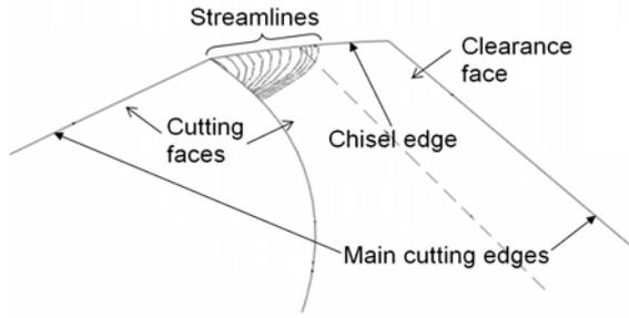
Fig. 7. Streamlines for a material point from the chisel edge to the flute.
