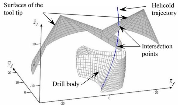
**Fig. 3.** Biconical machining— construction of the intersection between the tip and the body of the drill.
