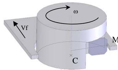
Fig. 3. Tool and machining configuration for second test series.
