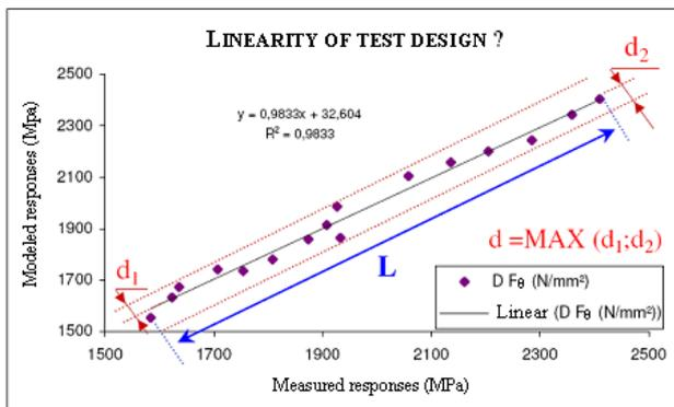
Fig. 9. Test design linearity validation.
