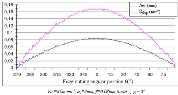
Fig. 7. Example of real instantaneous radial feed and chip section.
