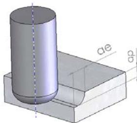
Fig. 2. Tool and machining configuration of first test series.
