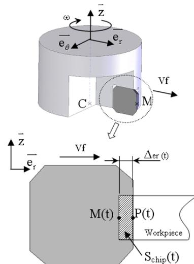
Fig. 6. Real instantaneous undeformed chip section.
