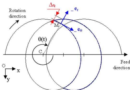
Fig. 4. Path of a peripheral point of the mill.
