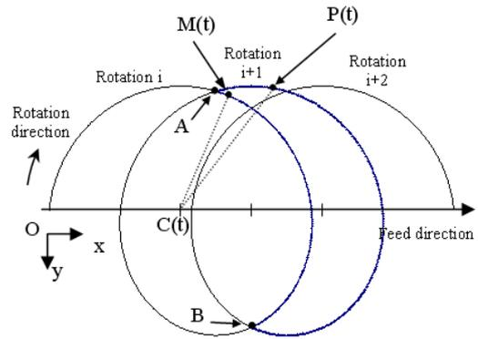
Fig. 5. Parameters for undeformed chip section calculus.
