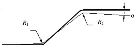
Fig. 3. Springback parameters.
