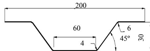
Fig. 1. Geometry of the parts.
