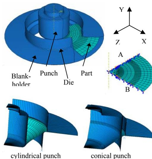
Fig. 2. Geometry of the model used in simulation.
