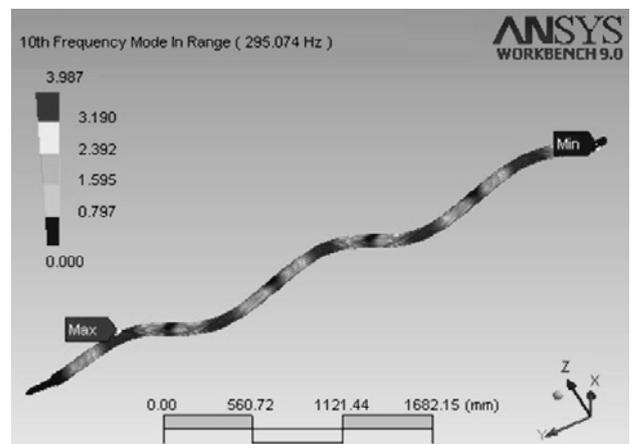
Fig. 8. 10<sup>th</sup> Frequency mode for the screw-drive.
