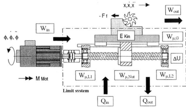
$M_{Mot}$  – torques moment;  $F_f$  – friction force;  $W_{in}$ ,  $W_{out}$  – work feed in and out;  $Q_{in}$ ,  $Q_{out}$  – warm volume in and out;  $E_{kin}$  – kinematic energy;  $\Delta U$  – difference of internal energy;  $W_{\mu,G}$  – mechanical work in guide;  $W_{\mu,L1}$  – mechanical work in warehouses of the screw (L1);  $W_{\mu,Nut}$  – mechanical work in nut;  $W_{\mu,L2}$  – mechanical work in warehouses of the screw (L2).
