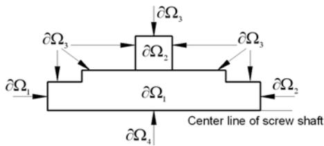
$\partial\Omega_1, \partial\Omega_2$  - constant temperature boundary;  $\partial\Omega_3$  - convective heat transfer boundary;  $\partial\Omega_4$  - adiabatic boundary;
