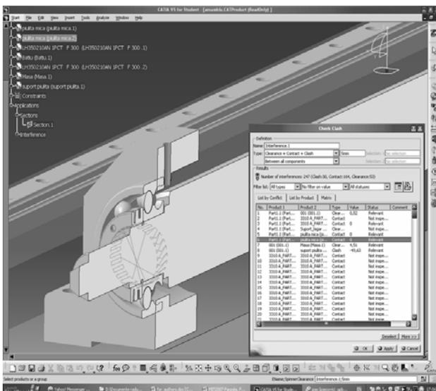
Fig. 3. Space analysis of the 3D model.
