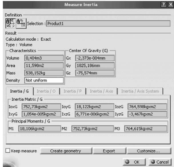
Fig. 4. CATIA inertia measurement tool.
