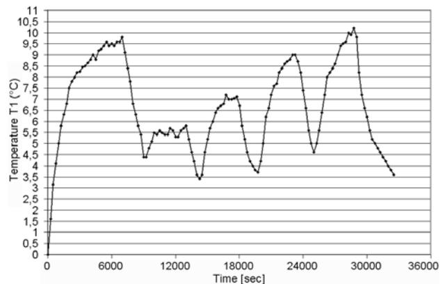
**Fig. 14.** Temperature profile of the front bearing ( $T_1$ ) during the thermal displacement measurement.
