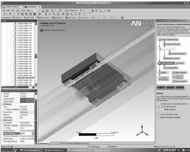
Fig. 6. Contact generation in ANSYS workbench.
