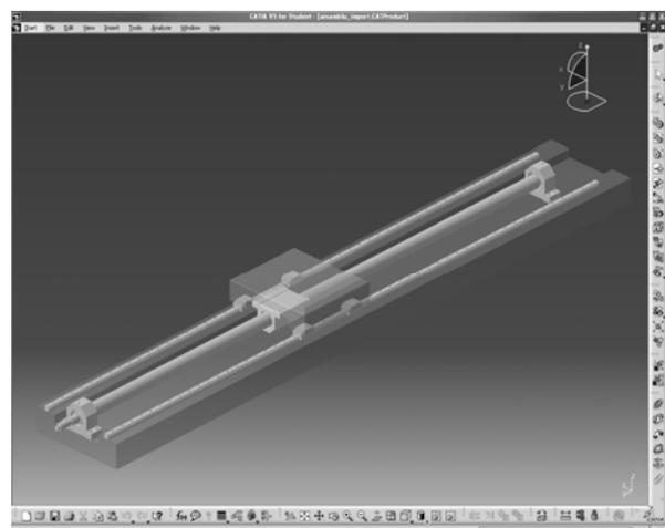
Fig. 1. 3D CAD model of the feed drive.
