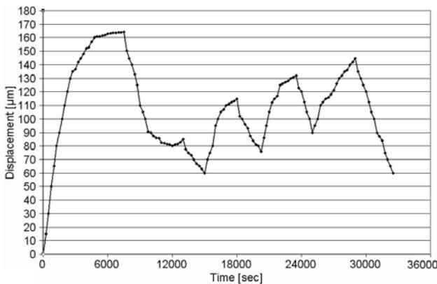
**Fig. 17.** Thermal displacement profile of the end of the ball screw.
