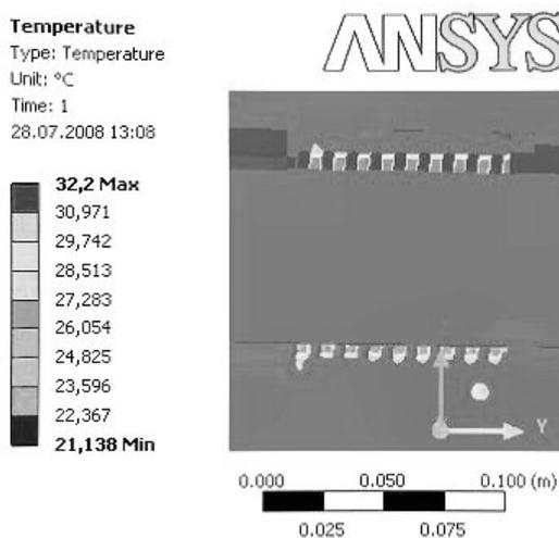
**Fig. 18.** Temperature profile of the nut ( $T_2$ ).
