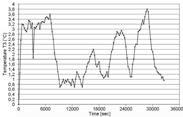
**Fig. 16.** Temperature profile of the rear bearing ( $T_3$ ) during the thermal displacement measurement.
