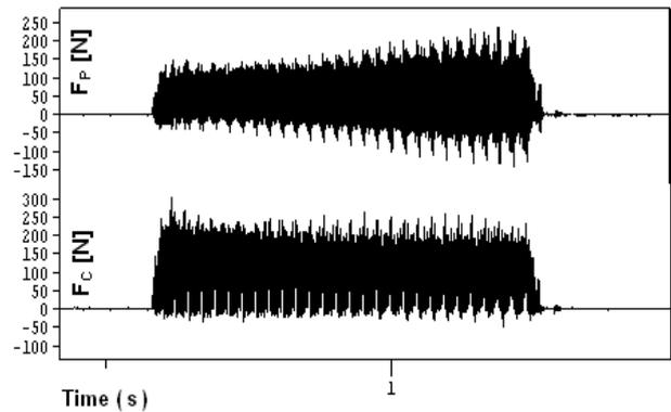
**Fig. 6.** Signal components of cutting force  $F_c$  and  $F_p$  for  $V_w' = 1\,500 \text{ mm}^3$  during grinding  $\text{Al}_2\text{O}_3$  at  $a_p = 0.03 \text{ mm}$ , wheel diameter 195 mm [1].
