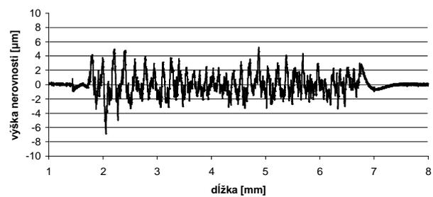
Fig. 10. Record of surface roughness for  $V_w' = 30$  mm<sup>3</sup> wheel  $Al_2O_3$  ( $D = 195$ mm), at  $a_p = 0.03$  mm [1].
