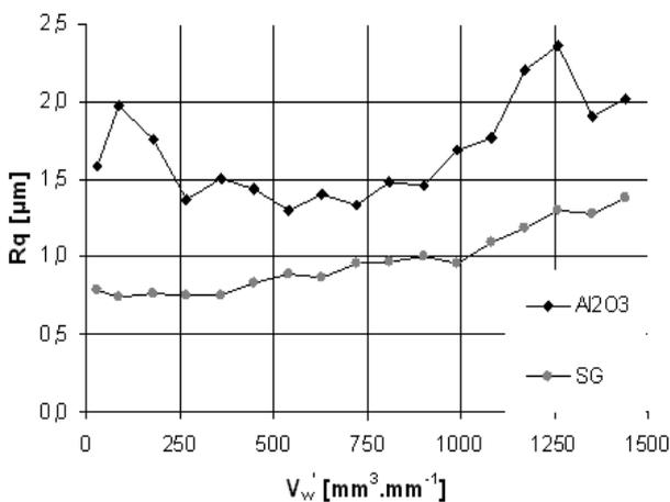
Fig. 14.  $V_w'$  influence on surface roughness  $R_q$  at  $a_p = 0.03$  mm.
