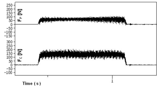
**Fig. 7.** Signal components of cutting force  $F_c$  and  $F_p$  for  $V_w' = 1\,500 \text{ mm}^3$  during grinding at  $a_p = 0.03 \text{ mm}$ , SG wheel diameter 195 mm [1].
