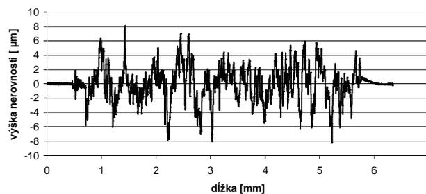
Fig. 11. Record of surface roughness for  $V_w' = 1$  180 mm<sup>3</sup> wheel  $Al_2O_3$  ( $D = 195$  mm), at  $a_p = 0.03$  mm [1].
