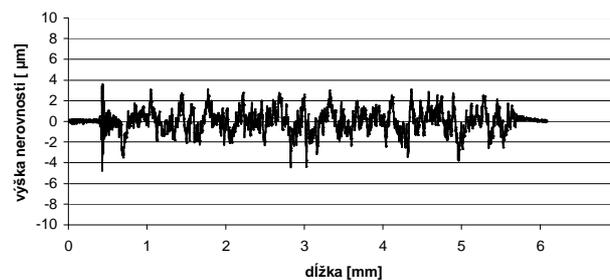
Fig. 12. Record of surface roughness for  $V_w' = 1$  180 mm<sup>3</sup> wheel SG ( $D = 195$  mm), at  $a_p = 0.03$  mm [1].
