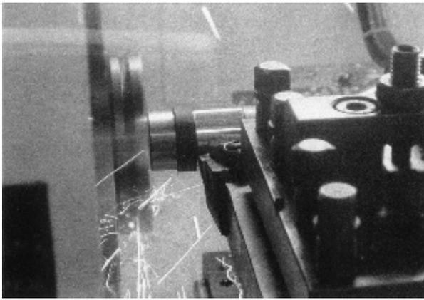
**Fig. 4.** Hard turning of the test sample of an tool with CA-estate CC6050 on CNC lathe HARRISON Alpha 1300S.
