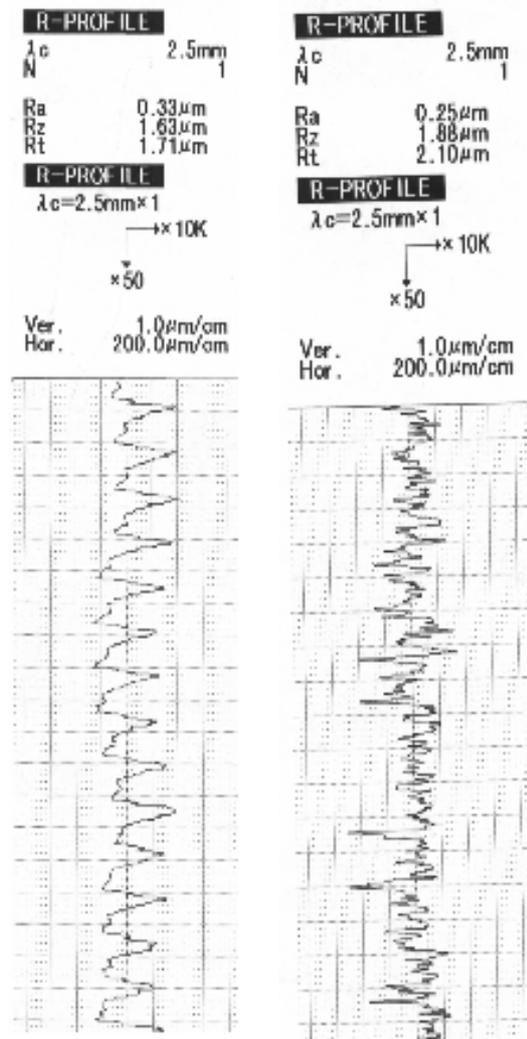
Fig. 16. Graphic recording of a surface roughness measurement for 102Cr6 dry turning (left) and cut (right).
