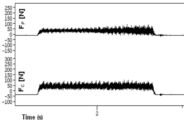
**Fig. 5.** Signal components of cutting force  $F_c$  and  $F_p$  for  $v_w' = \text{mm}^3 \cdot \text{mm}^{-1}$  in grinding  $\text{Al}_2\text{O}_3$  at  $a_p = 0.03 \text{ mm}$ , wheel diameter 195 mm [1].
