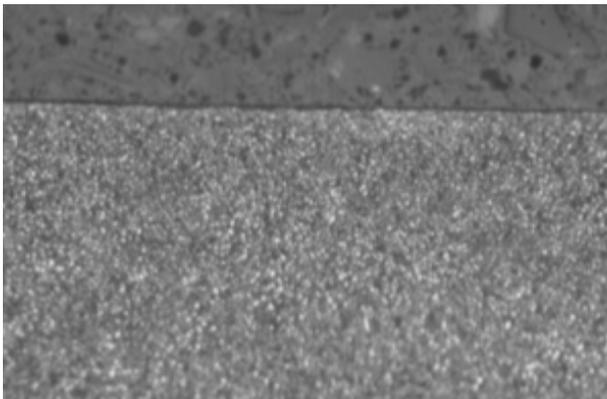
Fig. 2. Microstructure of surface layers of steel 102Cr6 after grinding, etched Nital 3% magnification 500× [2].
