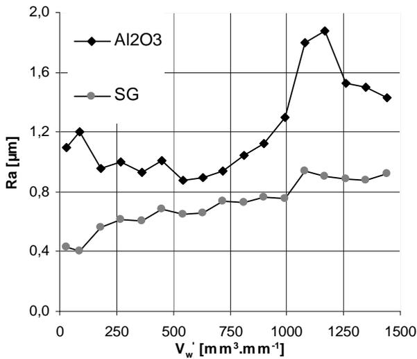
Fig. 13.  $V_w'$  influence on surface roughness  $R_a$  at  $a_p = 0.03$  mm without sparks.
