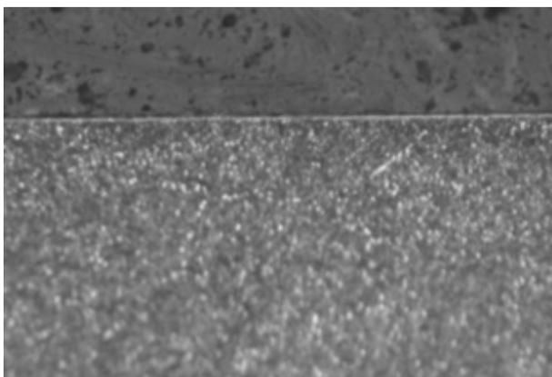
Fig. 3. Microstructure of surface layers of steel 102Cr6 after hard turning dry etched Nital 3% 500× magnification [2].
