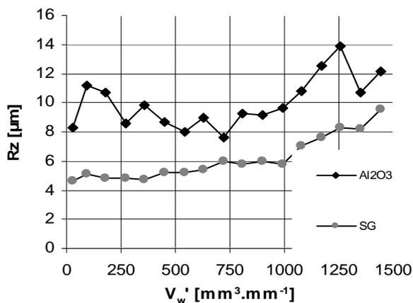
Fig. 15.  $V_w'$  influence on surface roughness  $R_z$  at  $a_p = 0.03$  mm.
