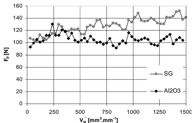
**Fig. 8.** Influence of  $V_w'$  on the static component of force  $F_p$  at  $a_p = 0.03 \text{ mm}$  [1].
