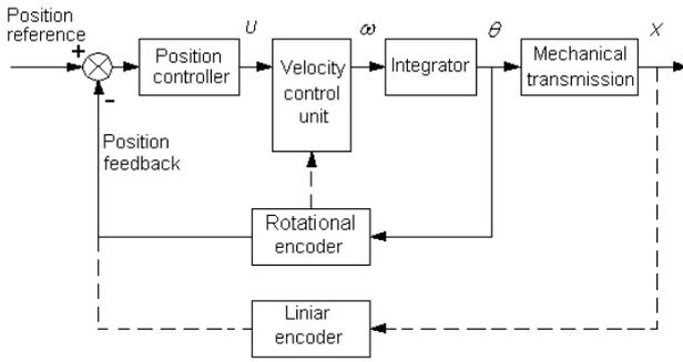
Fig. 5. Schematic structure of a position control servo system.
