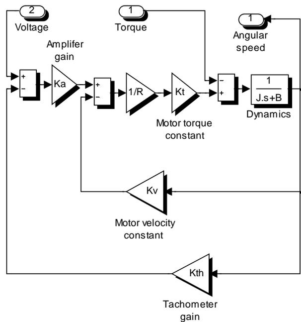
Fig. 8. The velocity loop subsystem.
