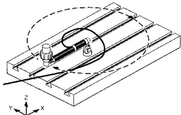
Fig. 1. The ballbar system.
