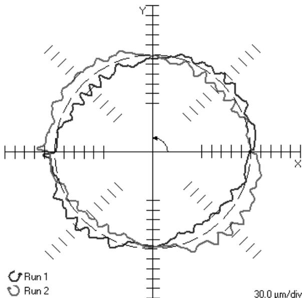
**Fig. 11.** The measurement after compensating the reversal spikes on X-axis.
