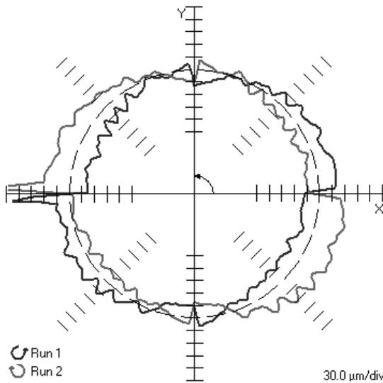
Fig. 3. The second measurement after a mechanical adjustment of the encoder mountings.
