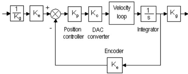
Fig. 6. The block diagram of the position control system.
