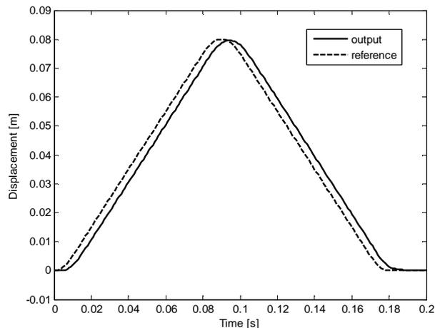
**Fig. 10.** Position output – compensated system.
