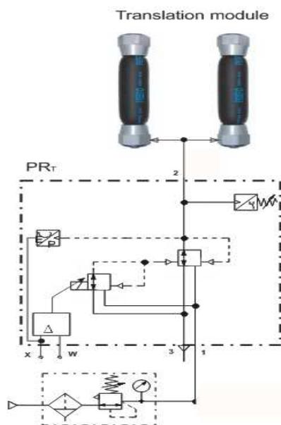
**Fig. 11.** Pneumatic actuation diagram.
