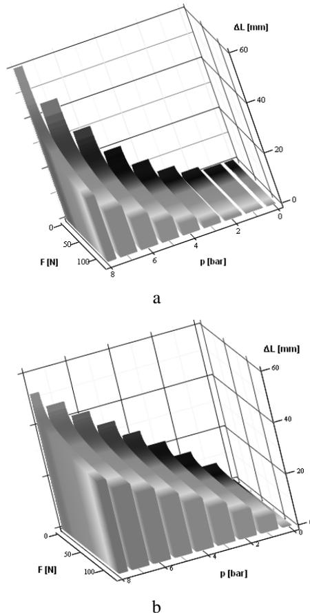
**Fig. 10.**  $\Delta L = f(p, F)$ : *a* – inflation of the pneumatic muscles; *b* – deflation of the pneumatic muscles.
