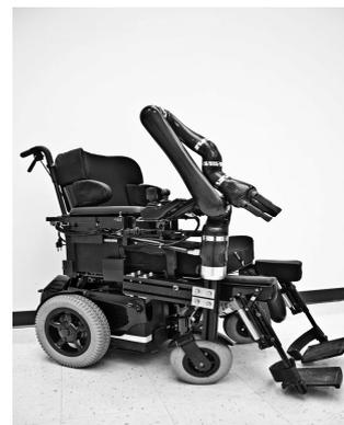
Fig. 1. Robotic arm on a wheelchair (JACO).
