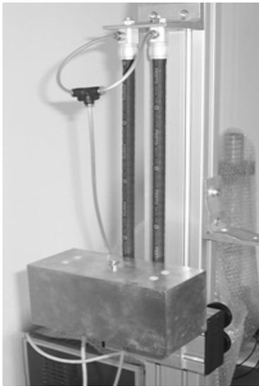
Fig. 6. Construction of the translation module.
