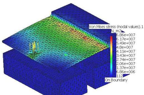
Fig. 8. Von Mises stresses of the thin wall in the middle area, four forces of 25 N each, wall thin of 1.45 mm.
