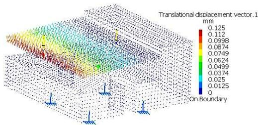
Fig. 5. Deformations of the thin wall in the middle area, two forces of 145 N each, wall thin of 2.5 mm.
