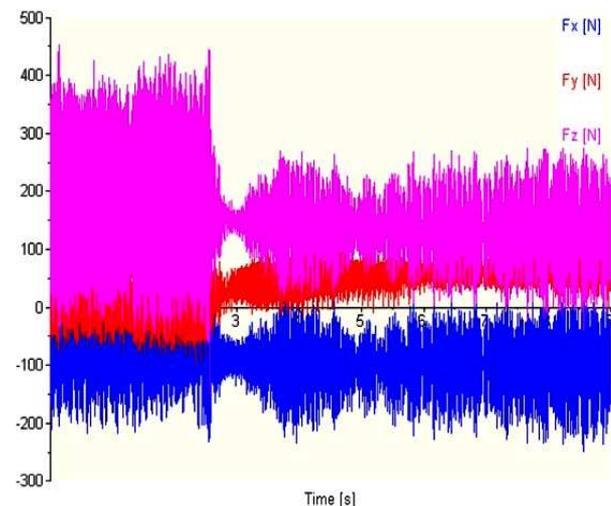
Fig. 12. Cutting forces at end milling, roughing pass.
