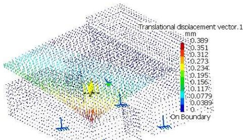
Fig. 7. Deformations of the thin wall at one of the ends, four forces of 25 N each, wall thin of 1.45 mm.
