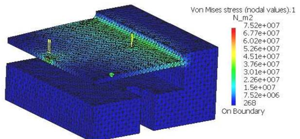
Fig. 4. Von Mises stresses of the thin wall ( ) in the middle area, two forces of 145 N each, wall thin of 2.5 mm.
