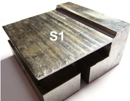
Fig. 16. Machined surface aspect after finishing milling.
