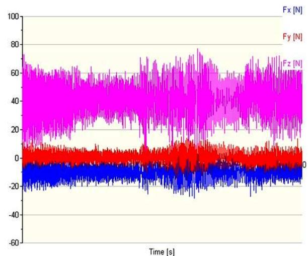
Fig. 17. Cutting forces at milling with an end mill of  $D_c = 8$  mm diameter.
