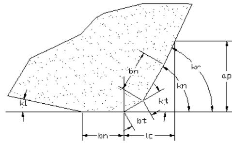
Fig. 3. Contact length between cutting edge and workpiece.
