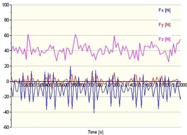
**Fig. 18.** Cutting forces for 0.02 s at milling with an end mill of  $D_c=8$  mm diameter.
