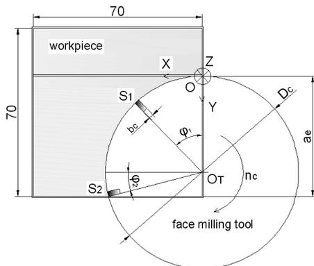
Fig. 2. Positions of the cutting spots.
