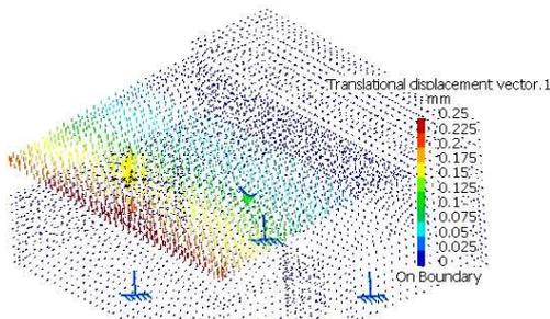
Fig. 9. Deformations of the thin wall in the middle area, four forces of 25 N each, wall thin of 1.45 mm.
