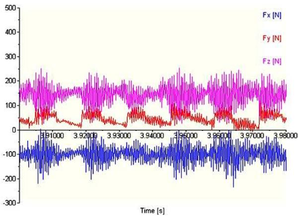
Fig. 13. Cutting force components on tool revolution (0.08 s).
