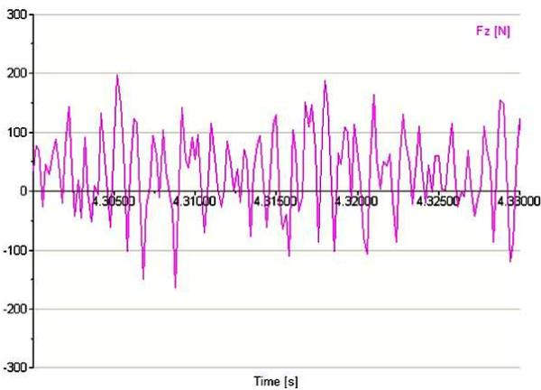
Fig. 14. Cutting force  $F_z$  on tool revolution, for the end mill with diameter  $D_c = 25$  mm.
