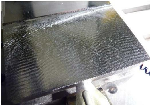
Fig. 15. Machined surface aspect after roughing end milling.
