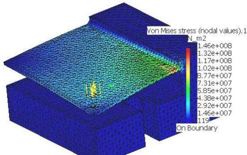
Fig. 6. Von Mises stresses of the thin wall at one of the ends, four forces of 25 N each, wall thin of 1.45 mm.
