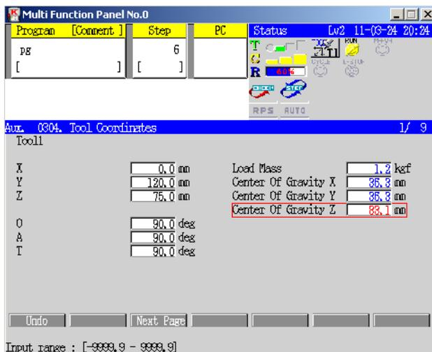
Fig. 12. Tool configuration data introduced in the Auxiliary Settings menu of the virtual teaching panel.
