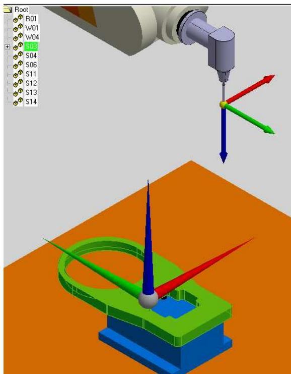
Fig. 8. The positioning of the axis systems attached to the part and to the end-effector.
