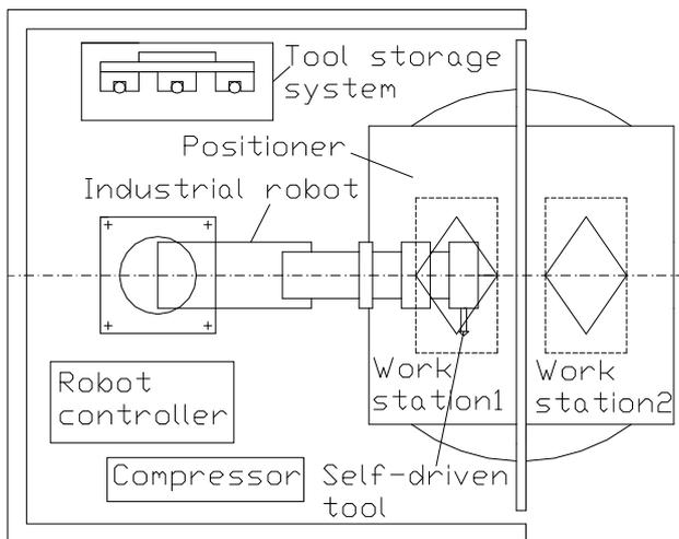
Fig. 2. The general structure of a first principle flexible manufacturing cell.
