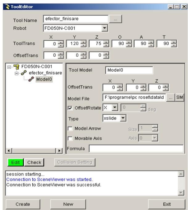
Fig. 10. Tool configuration using the Tool Editor module.
