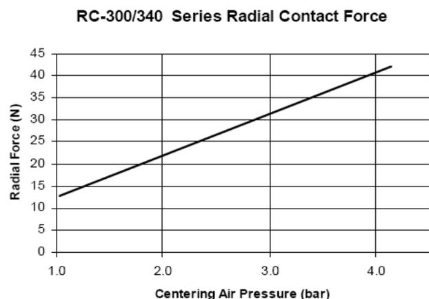
Fig. 13. RC-340 radial contact force-centering air pressure diagram.
