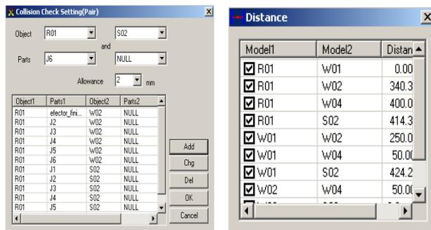
Fig. 6. The constraints between the cell components specified in the Display Model's Minimum Distance and Collision Check Setting tools.
