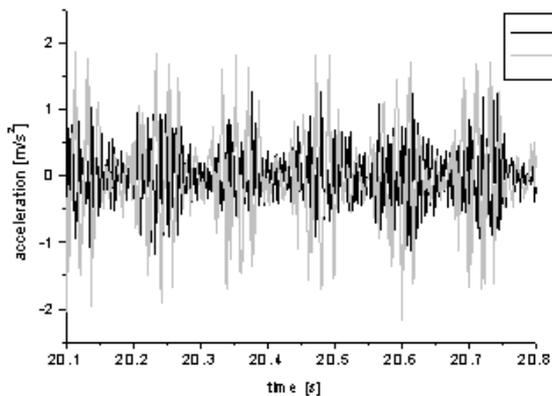
**Fig. 11.** Vibrations during milling process, when X and Y axis moving in the other direction.
