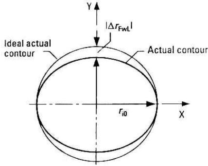
Fig. 3. Circular contour distortions due to amplitude errors.
