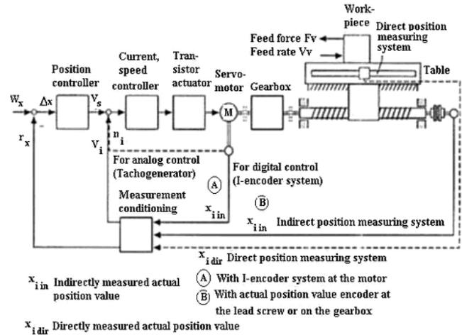
**Fig. 2.** Indirect and direct position measurement in the position control loop [5].
