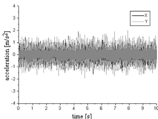
Fig. 8. Vibrations during finishing milling.
