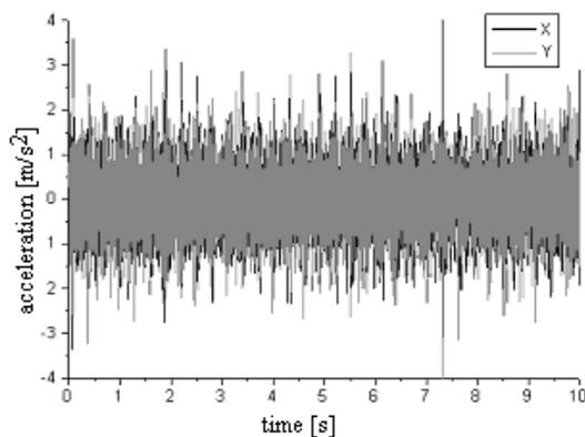
Fig. 7. Vibrations during roughing milling
