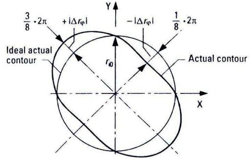
Fig. 4. Circular contour distortions due to phase error.
