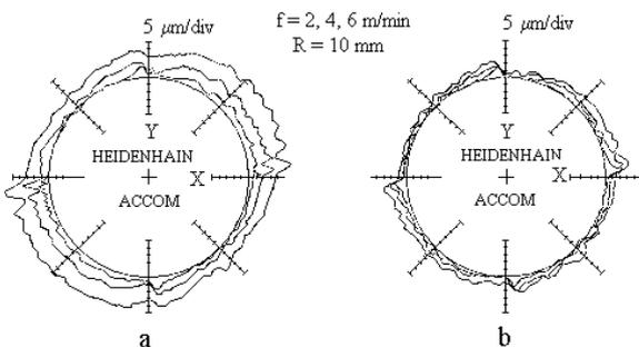
**Fig. 1.** Circular test of machining center a) position control with rotary encoder; b) position control with linear encoder.
