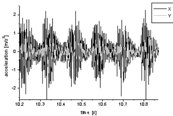
**Fig. 10.** Vibrations during milling process, when X and Y axis moving in one direction.
