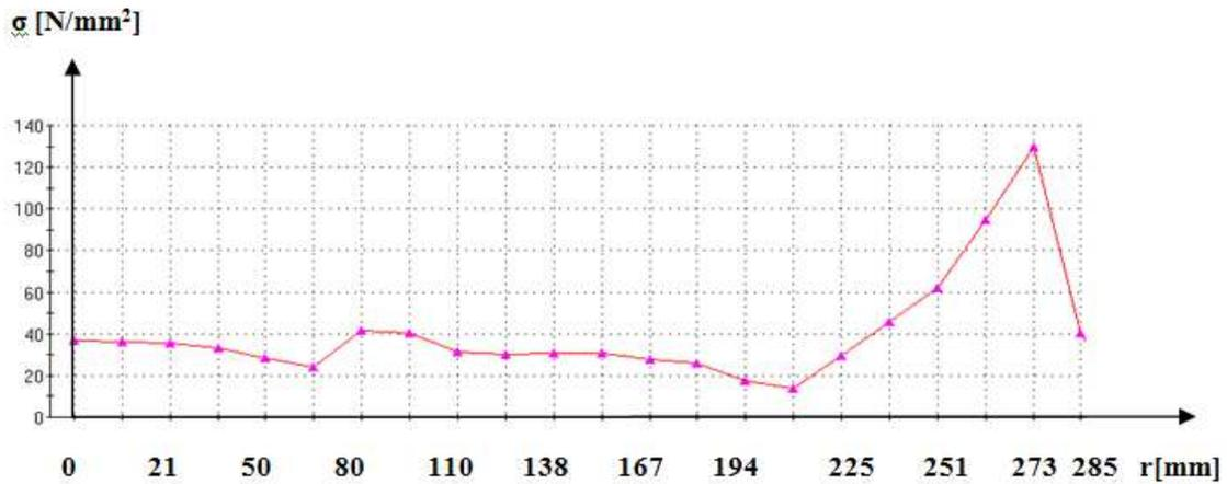
Fig. 9. Stresses of the fixed ribbed plate, at 0.3 MPa pressure.
