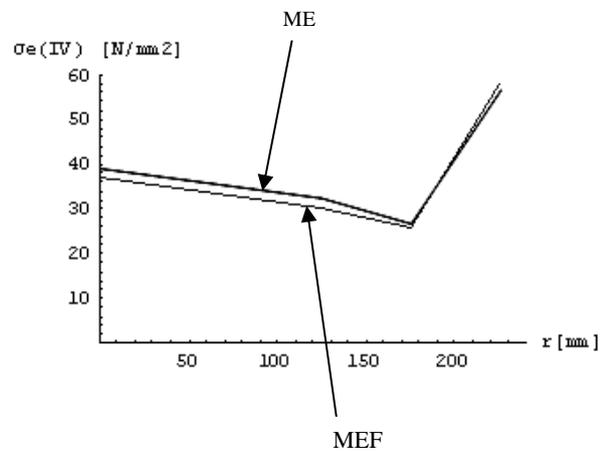
Fig. 11. The variation of the equivalent stresses which are calculated on the basis of the fourth resistance theory.
