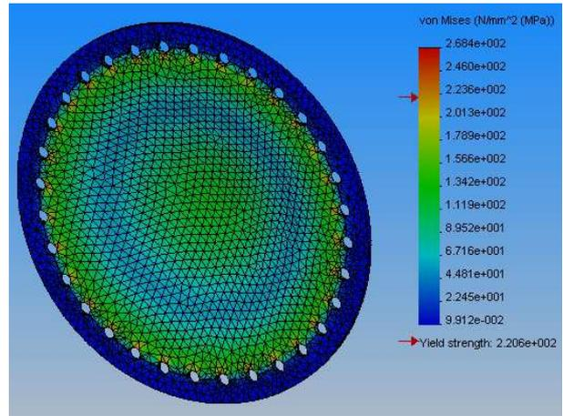
Fig. 2. Stresses of the fixed plane plate, at pressure 0.3 MPa.
