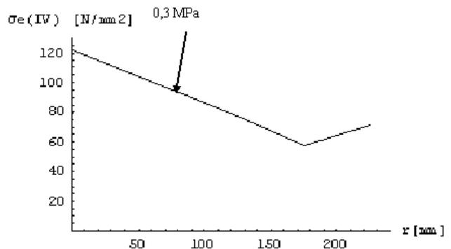
Fig. 6. The variation of the equivalent stresses which are calculated on the basis of the fourth resistance theory.
