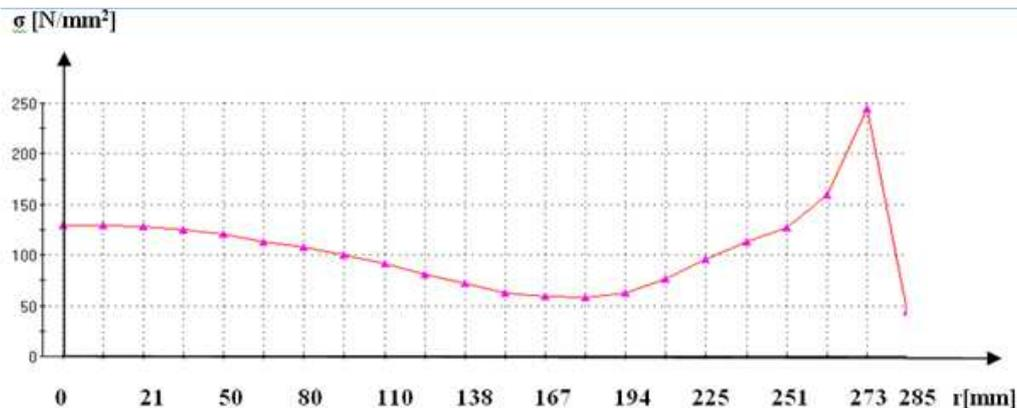
Fig. 3. Stresses of the fixed plane plate, at 0.3 MPa pressure.
