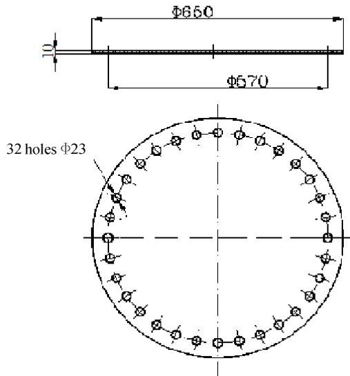
Fig. 1. Geometrical characteristics of the circular plane plate.
