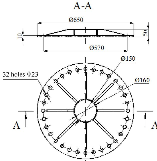
Fig. 7. Geometrical characteristics of the circular ribbed plate.
