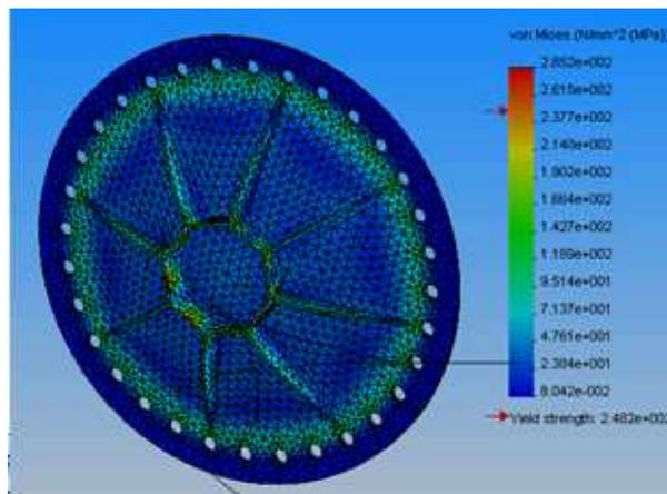
Fig. 8. Stresses of the fixed ribbed plate, at 0.3 MPa pressure.
